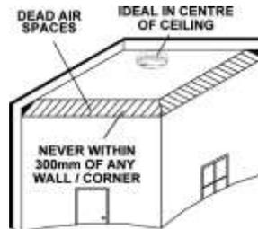
Alarms should be placed in accordance with the general guidelines shown in the diagram above. These recommendations are based on the problem of areas of "dead air" close to corners of rooms and apexes of ceilings, which could result in the prevention of heat reaching the heat detector
