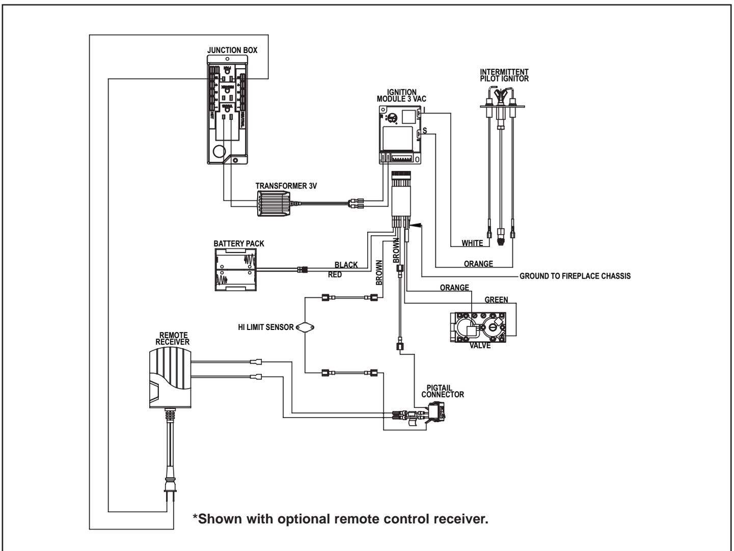
**Figure 10. Intermittent Pilot Ignition (IPI) Wiring Diagram**
