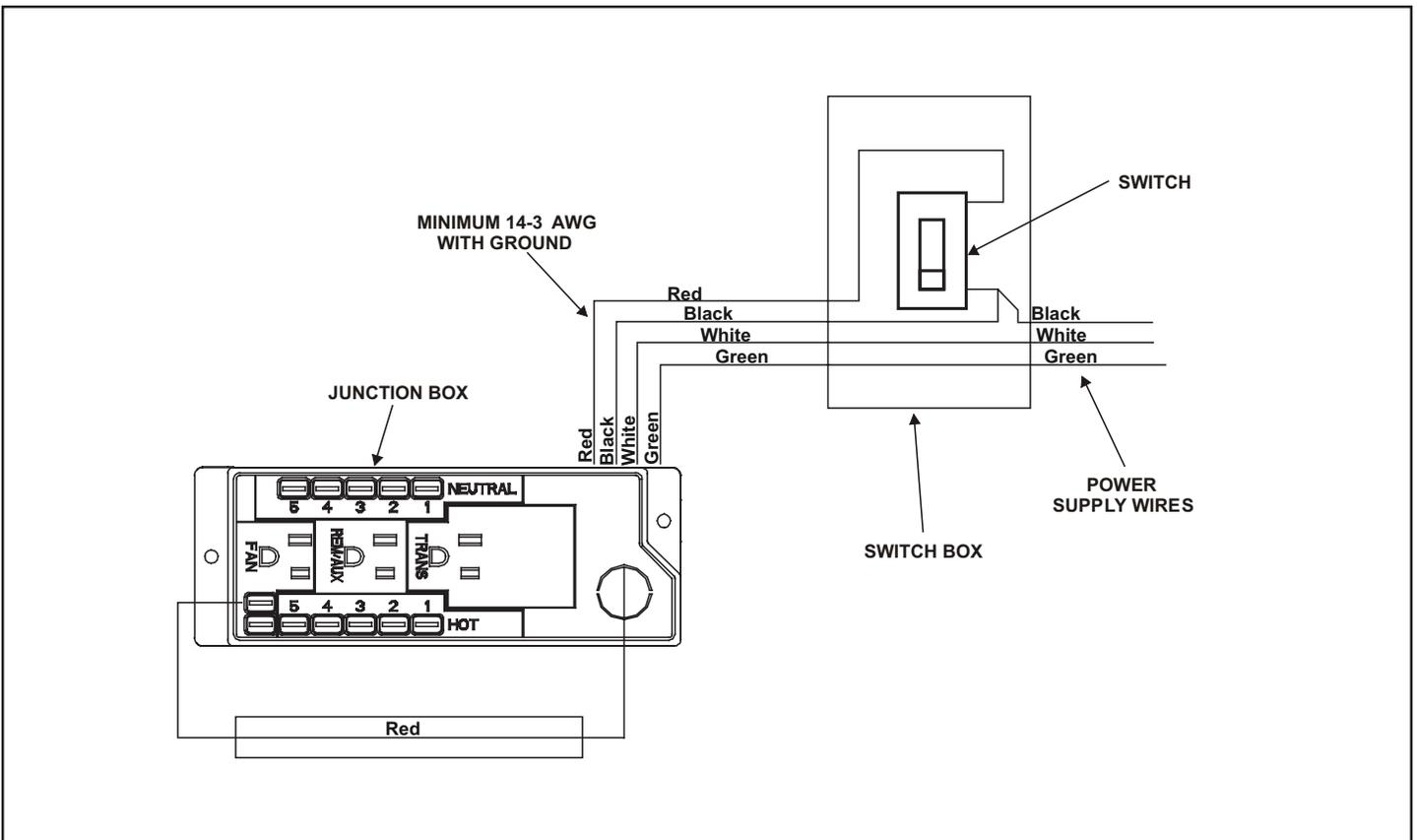
Figure 11. Junction Box Wired to Wall Switch
