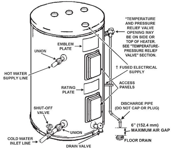
† ELECTRICAL CONNECTIONS MAY BE LOCATED ON THE TOP OR SIDE, REFER TO YOUR UNIT. ACTUAL MODEL AND ILLUSTRATION MAY VARY DEPENDENT ON MODEL CAPACITY AND TYPE. SOME MODELS HAVE ALTERNATE INLET, OUTLET AND T&P VALVE LOCATIONS. THESE ALTERNATE LOCATIONS ARE IDENTIFIED BY THE LABELING ON THE UNIT.
