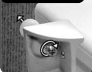
3. Attach the mounting brackets to the sides of the transceiver with the adjusting screw flanges facing the back of the flat surface.
