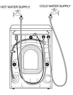
Before connecting the hoses, be sure to fit the black washers supplied as per diagram.
