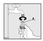
If only a cold water supply is available, connect the two hoses to a cold water outlet by means of a 'Y' connection piece.
