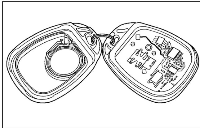
1. Insert a coin, or similar object, in the slot between the covers of the transmitter housing. Gently pry the transmitter apart.
