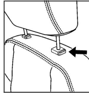
Pull the head restraint up to raise it. To lower the head restraint, press the button, located on the top of the seatback, and push the head restraint down.
