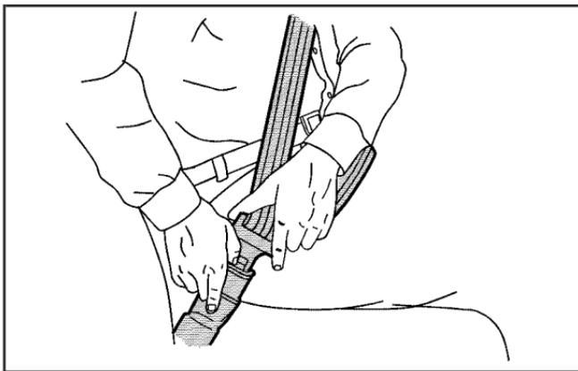
To unclash the belt, just push the button on the buckle. The belt should go back out of the way. When the safety belt is not in use, slide the latch plate up the safety belt webbing. The latch plate should rest on the stitching on the safety belt, near the guide loop on the side wall.
