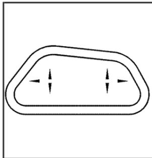
Your vehicle may have this feature. If it does, the six-way power seat control is located on the outboard side of the driver's seat. Your vehicle may also have a passenger's six-way power seat.
