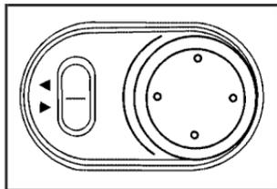
The outside power mirror controls are located on the driver's door armrest.
