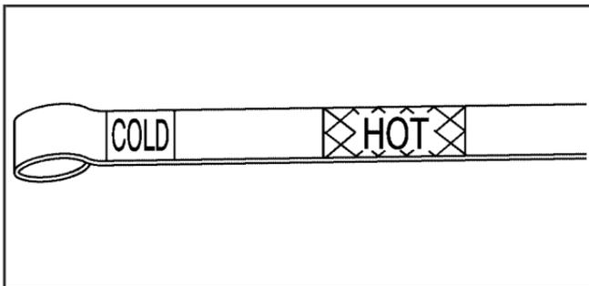
3. Check both sides of the dipstick, and read the lower level. The fluid level must be in the COLD area, below the cross-hatched area, for a cold check or in the HOT or cross-hatched area for a hot check. Be sure to keep the dipstick pointed down to get an accurate reading.
