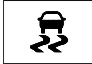
To turn the system off, press and release the TCS button located on the instrument panel.
