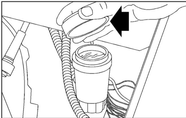
Refer to the Maintenance Schedule to determine how often you should check the fluid level in your clutch master cylinder reservoir and for the proper fluid. See *Recommended Fluids and Lubricants* on page 6-12.
