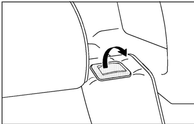
4. Lift the latch on top of the seatback and pull the seatback forward. Fold the seatback down until it is nearly flat.
