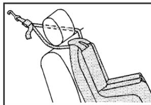
If the position you are using has a fixed head restraint and you are using a dual tether, route the tether around the head restraint.
