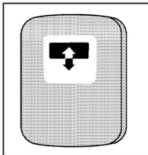
The switch used to operate the sunroof is located in the headliner.
