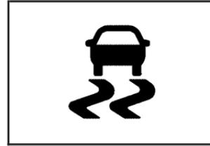
If you have the traction control system, this light will come on when the traction control system has been turned off.
