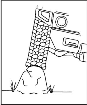
Do not straddle large rocks; drive over them, letting the tire cover the rock. The tread of the tire is thicker and tougher than the sidewall of the tire and is more resilient to impact than underbody components.
