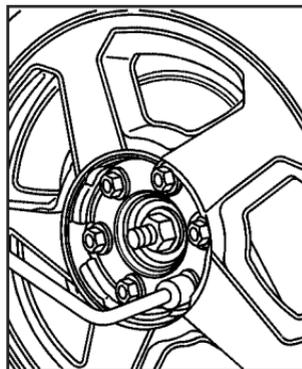
2. Use the wheel wrench to remove the wheel nuts securing the spare tire.
