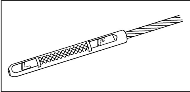
If the oil is below the cross-hatched area (L), you will need to add at least one quart/liter of oil. But you must use the right kind. This section explains what kind of oil to use. For engine oil crankcase capacity, see *Capacities and Specifications on page 5-100*.
