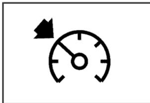
The cruise symbol on the instrument panel will illuminate when the cruise control is engaged.
