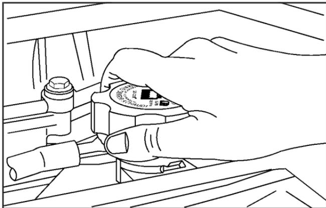
1. You can remove the radiator pressure cap when the cooling system, including the upper radiator hose, is no longer hot. Turn the pressure cap slowly counterclockwise about one full turn. If you hear a hiss, wait for that to stop. A hiss means there is still some pressure left.
