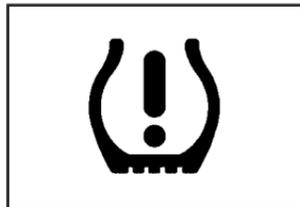
This light should come on briefly when you turn the ignition to ON. It will then come on only when a flat or low tire pressure condition exists.
