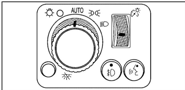
The control on the driver's side of your instrument panel operates the exterior lamps.
