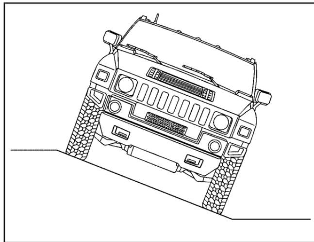
Also, your vehicle should be able to traverse a 40% (22 degrees) side slope at 6 mph (9.7 km/h) while fully loaded on high friction surfaces.
