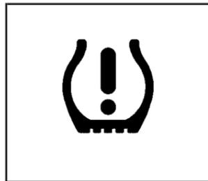
As an added safety feature, your vehicle has been equipped with a tire pressure monitoring system (TPMS) that illuminates a low tire pressure telltale when one or more of your tires is significantly under-inflated.
