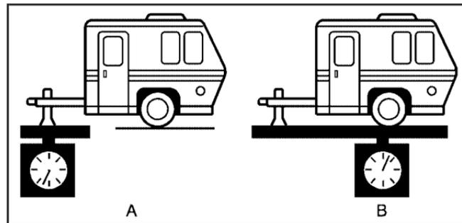
The trailer tongue weight (A) should be 10 percent to 15 percent of the total loaded trailer weight (B), up to a maximum of 500 lbs (227 kg) with a weight carrying hitch or a weight distributing hitch.
