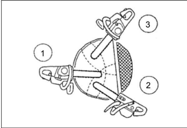
To fell big trees with a diameter exceeding twice the bar length, start the notching cuts from one side and draw the saw through to the other side of the notch. Start the back cut on one side of the tree, pivoting the saw through to form the desired hinge on that side. Then remove the saw for the second cut. Insert the saw in the first cut, very carefully so as not to cause kickback. The final cut is made by drawing the saw forward in the cut to reach the hinge.
