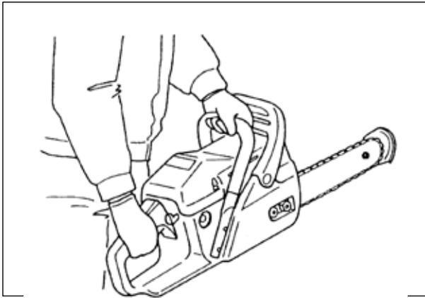
The accepted way to hold the saw is to stand to the left of the saw with your left hand on the front handlebar and your right hand on the rear handle so you can operate the throttle trigger with your right index finger. Before attempting to fell a tree, cut some small logs or limbs. Become thoroughly familiar with the controls and the responses of the saw.
