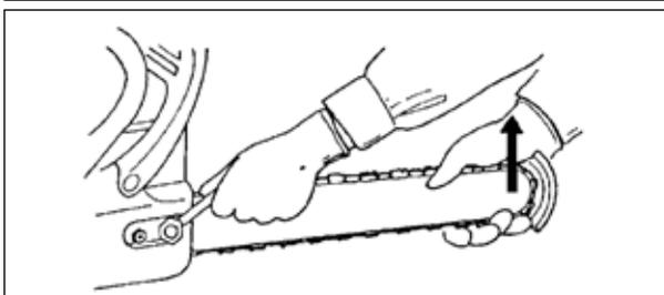
4. Unlock the chain brake, and mount guide bar on studs and slide toward clutch to make saw chain installation easier. Install chain with cutters on top of guide bar facing forward.
