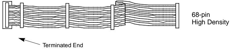
SCSI Cable for Internal Connections
