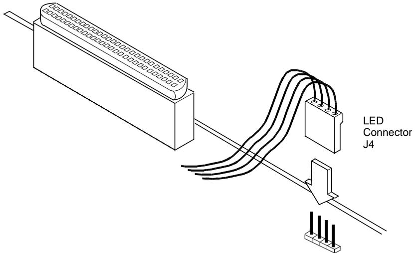
Some LED cables have only two wires. In this case, place the connector on one end or the other of J4. If the LED does not light during SCSI bus activity from this host adapter, you may have to rotate the LED cable connector 180° on J4.
