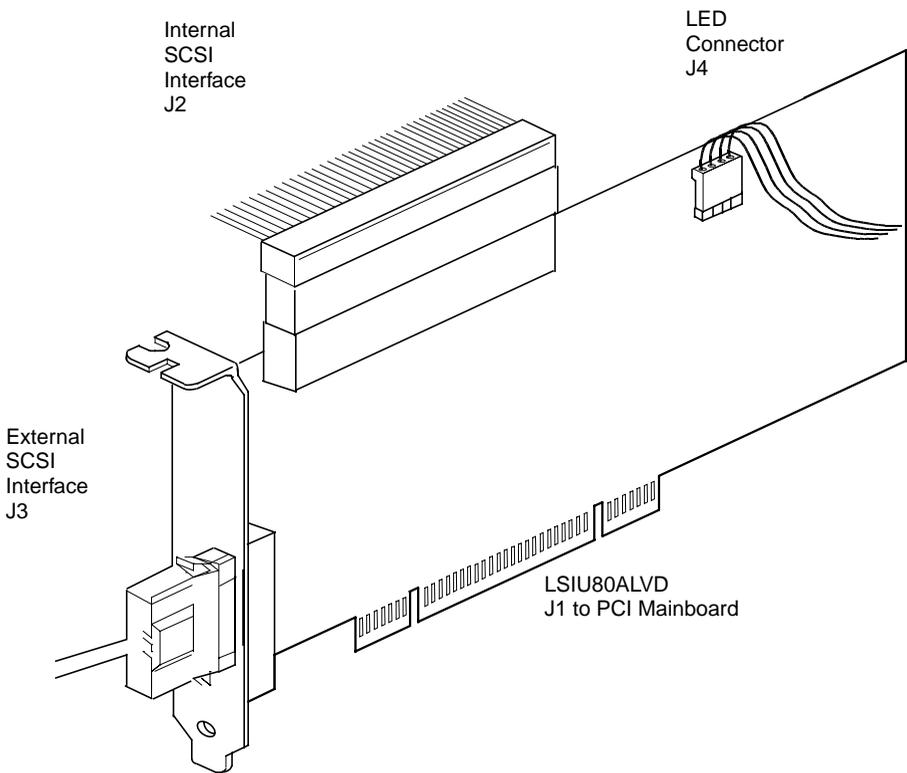
Step 6. Carefully insert edge connector J1 (see [Figure 2.1](#)) of the host adapter into the PCI slot. Make sure the edge connector is properly aligned before pressing the board into place as shown in [Figure 2.2](#).
