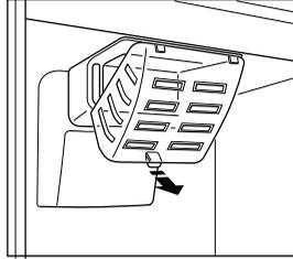
press on the rear hook and at the same time slide the cover in the direction indicated by the arrow. Unscrew the bulb and replace it with one of the same power (the maximum power is shown on the light diffuser) available from your nearest Service Force Centre. Replace the light cover by sliding it into its original position.
