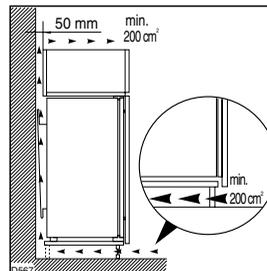
Furthermore, it is necessary that the cabinet has a ventilation recess with the following dimensions:
