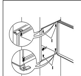
Apply the sealing strip pushing it between the refrigerator and the adjacent cabinet.
