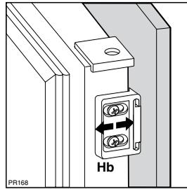
Fix cover (Hd) on guide (Hb) until it clips into place.
