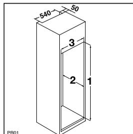
Make sure that a distance of 44 mm is maintained in the lower part between the kitchen furniture and the border of the appliance.
