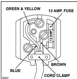
Connect the Green and Yellow (earth) wire to the terminal in the plug which is marked with the letter «E» or the earth symbol
