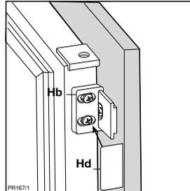
Fix the appliance to the side of the kitchen unit, fit the bracket (E) and (F), adjust the distance, and fix using the screws (as in figure). Fit the cover (D).
