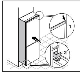
Fasten the appliance with 4 screws provided in the kit included with the appliance.
