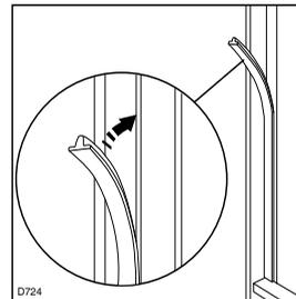
From the plastic cover (E), which is used to cover the hinge with the pivot pin, you must take away the part as indicated in the drawing.
