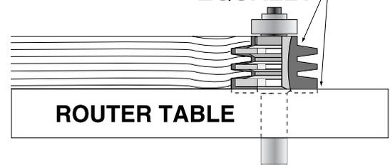
**Helpful hint:** For each paired joint, make your first cut with the marked face up. To make the matching cut on your second piece of lumber, turn it over so the marked face is down. When you have completed your second
