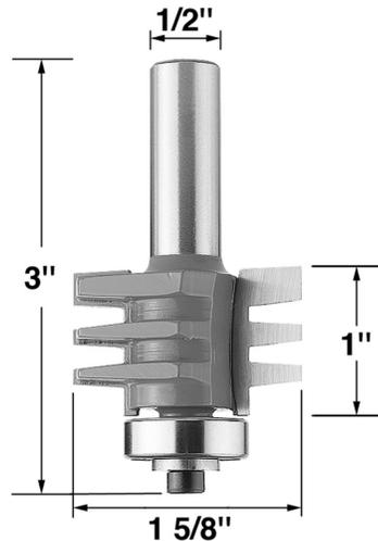
The Model C1367 Finger Joint Bit is designed specifically for creating strong, tight-fitting end joints in  $\frac{3}{4}$ " thick stock. The bit features tough carbide cutting surfaces and a ball-bearing roller guide. This bit can be used in either a hand-held router or in a router table. For best results, we recommend using a router rated at a minimum of 1 horsepower, mounted in a router table to ensure maximum safety and efficiency.
