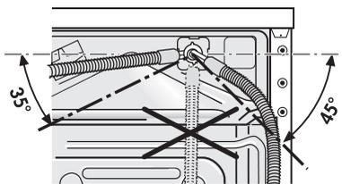
2. Connect the hose with the straight connection to a water tap with a screw thread of R 3/4 (inches).
