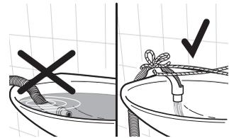
– When hooked into a wash-basin or a bath tub the drainage hose must be protected from slipping out of place by the supplied slip-on elbow. Otherwise the repelling power of the draining water can press the hose out of the sink.
