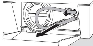
**4.** Place the collecting vessel underneath.
