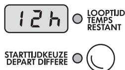
If *19h* is displayed and you press again, the run time of the set washing program (display in minutes, e. g. *125*) appears. In this state, the delay timer is not set.
