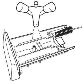
7. Use a brush to clean the entire rinsing-in part of the washing machine, especially the nozzles on the top side of the rinsing-in chamber.
