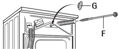
**Attention!** Push in the plug cap so firmly that it engages in the rear panel (this protects the inside of the unit against splash water).
