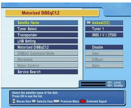
To use the DiSEqC 1.2 protocol, select the Installation > Motorized DiSEqC 1.2 menu. You should see a screen like the left figure.
