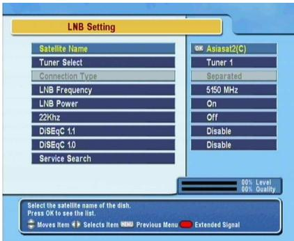
Select the Installation > LNB Setting menu to configure the LNB settings. You should see a screen like the left figure.
