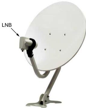
The LNB (Low Noise Block converter) is used to take a wide band of relatively high frequencies, amplify and convert them to similar signals that is carried at a much lower frequency, which is called Intermediate Frequency (IF).
