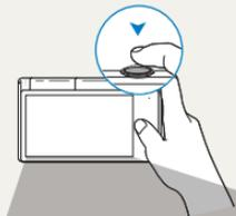
Half-press **[Shutter]** to adjust the focus. The camera adjusts the focus and exposure automatically.
