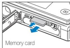
Push the card gently until it disengages from the camera, and then pull it out of the slot.
