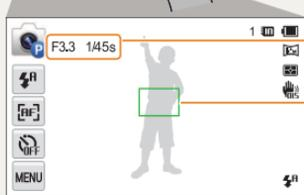
The camera sets the aperture value and shutter speed automatically.
