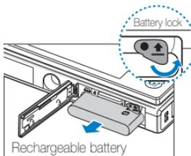
Push the lock up to release the battery.
