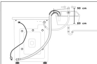
In a sink drain pipe branch
