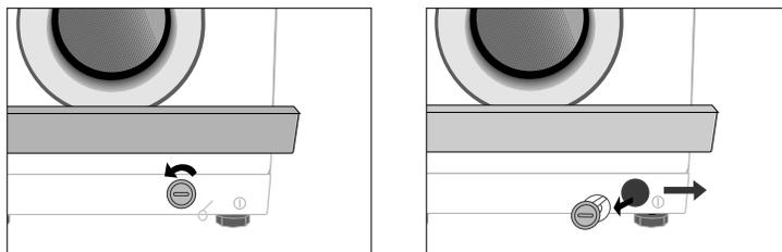
4. Wash any dirt or other material from the filter. Make sure the drain pump propeller behind the filter is not blocked. Replace the filter cap.
