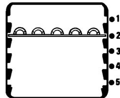
You can slot the oven shelves into any of five positions in the main oven and any of two positions in the top oven.
