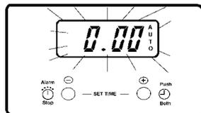
Press buttons (1) and (2) together. Release buttons, 0.00 will appear in the display as Fig. 2. **Within 5 seconds** press button (2), 12.00 will show in the display as Fig. 3.
