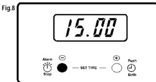
To return the timer to manual press button (1) again. See Fig. 8. If using the main oven it will come on again once button (1) has been depressed. When cooking is complete remove food and turn OFF oven temperature control.
