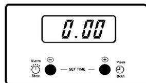
**Within 5 seconds** press and hold either button (1) to decrease or button (2) to increase the time until the correct time of day on the 24 hour clock is reached, e.g.14.30. See Fig. 4.
