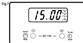
To stop the sound press button (1). The display will stop flashing and show the time of day, e.g. 15.00.
