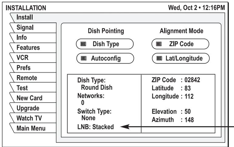
3. If the LNB type is set to “Stacked,” you do not need to change the setting. A different problem is causing the program guide not to load. Please call KVH Technical Support at 401-847-3327 (or e-mail [techs@kvh.com](mailto:techs@kvh.com)) for assistance.
