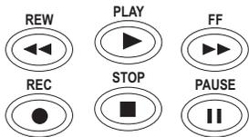
Use the VCR control buttons to operate your VCR or DVD player (the VCR component button must be selected first). *The remote control must be programmed to operate your VCR/DVD player for the VCR control buttons to work (see Section 3-3, "Programming the Remote Control to Operate Other Components," on page 3.10).*
