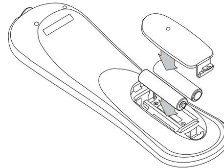
2. Insert two AAA batteries as shown, observing the correct polarity.
