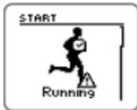
1. Start by pressing OK. The training computer enters pre-training mode and starts searching for the sensor signals. If a sensor signal is not found, the display will show a triangle with an exclamation mark. The check mark indicates that the sensor signal is found. Select the sport for the training session by browsing with the UP/DOWN buttons.
