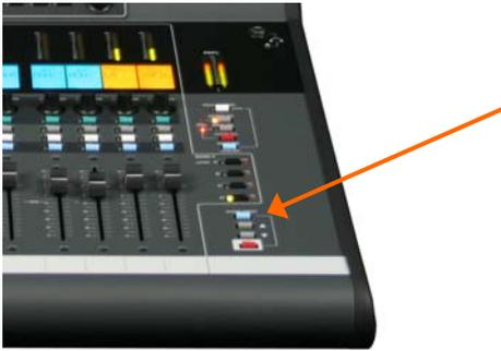
**Scene Recall Safes** lets you make selected input channels and mix masters 'safe' so that their parameters are not overwritten when a Scene is recalled. Hold down the **SCENE SAFES** key and press the strip **MIX** keys on channels you want to make safe. The **SAFE** icon in the strip LCDs turns on for channels made safe.
