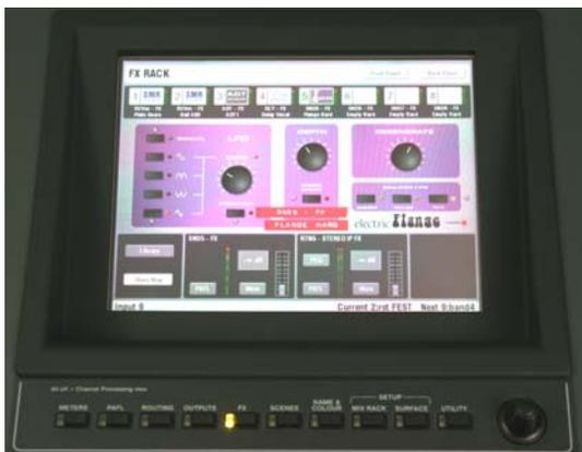
The TouchScreen provides access to the FX, setup and utility functions and presents an alternative graphical view of the channel processing parameters.
