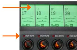
Start with the **DCA master fader** set to '0' normal position. In this position the assigned channel levels are unaffected by the master. Raise the master to boost the assigned channel levels by up to +10dB. Lower the master to reduce the levels to fully off.
