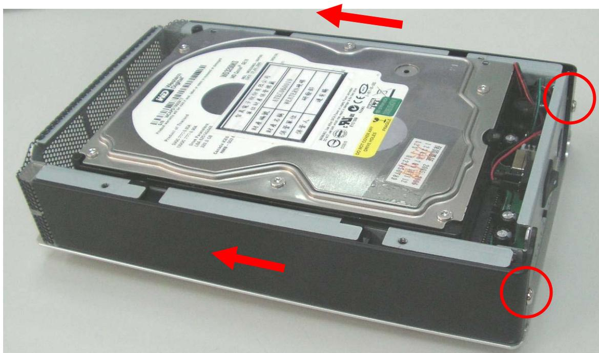
**STEP6:** Replace the aluminum cover back and tight up 4 screws.
