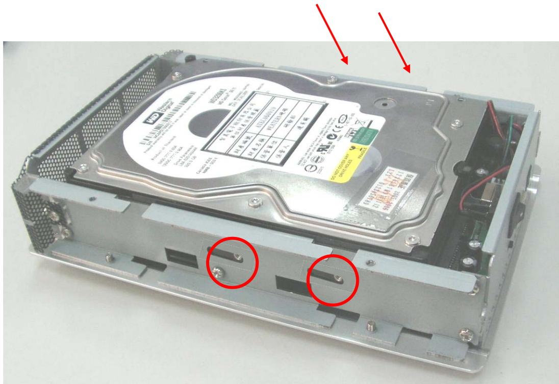
**STEP5:** Reassemble two side plates back to the enclosure and fix the screws.
