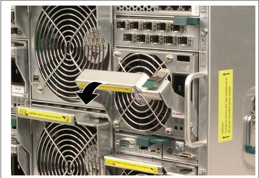
Figure 78: Removing the power supply unit
