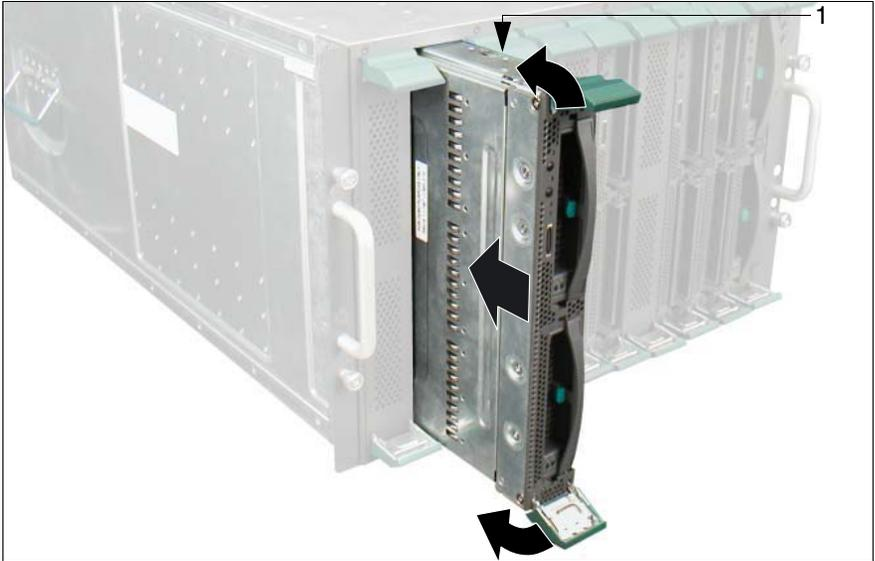
Figure 32: Inserting the server blade
