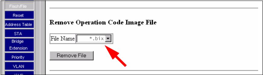
Figure 24: Removing an operation code image file
