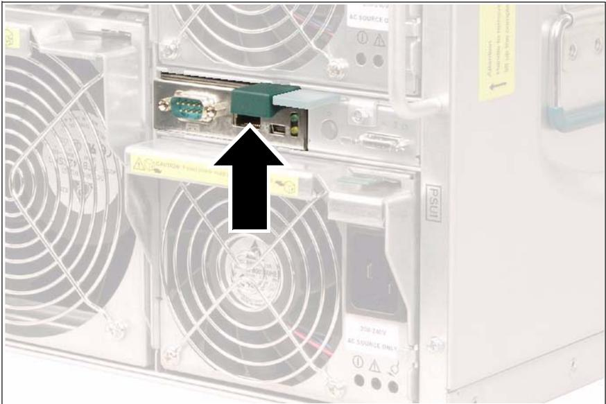
Figure 62: Disengaging the management blade
