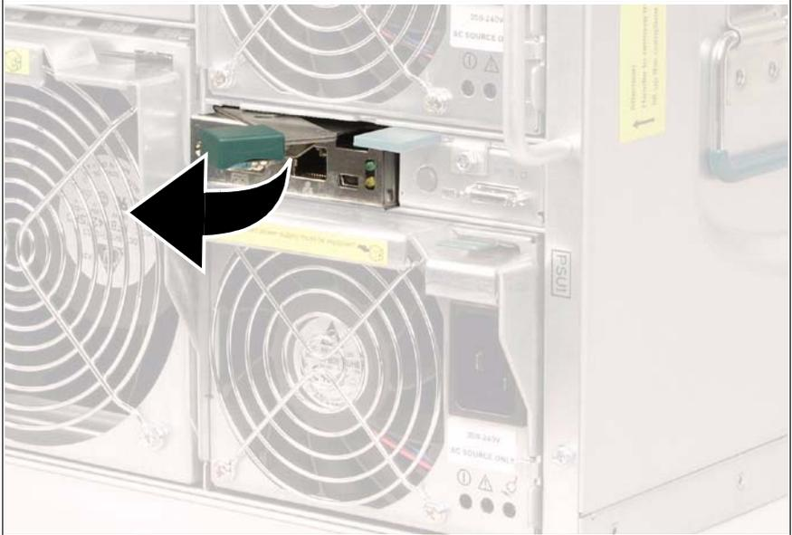
Figure 63: Disengaging the management blade
