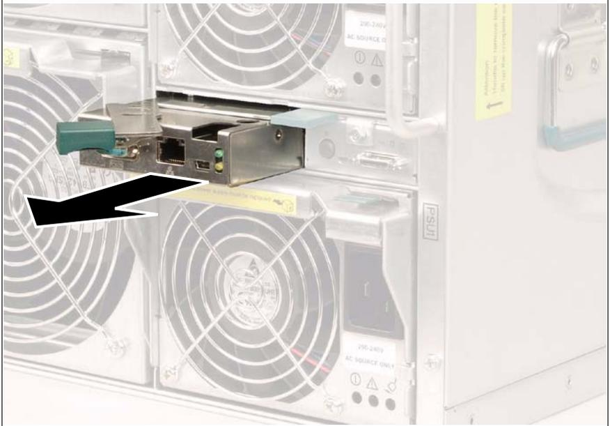
Figure 64: Removing the management blade
