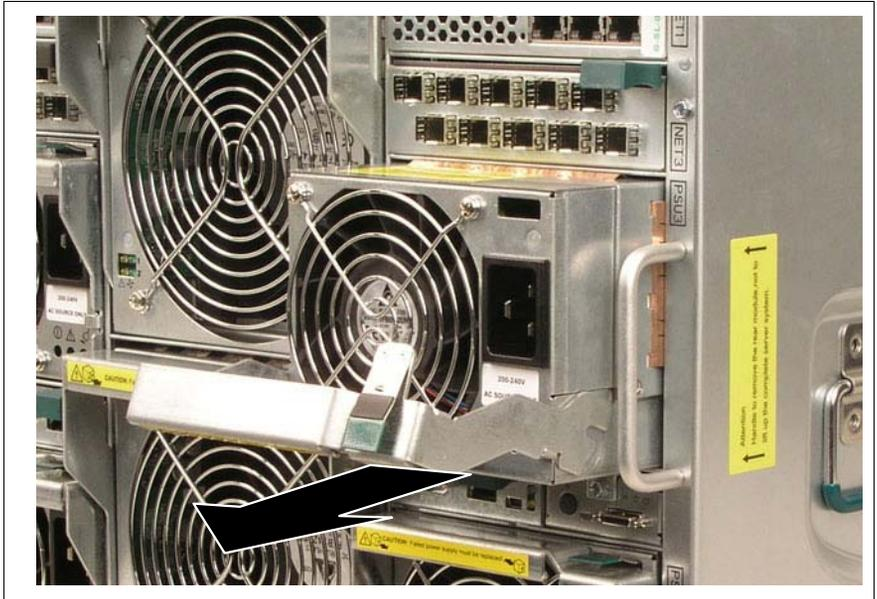
Figure 79: Removing the PSU
