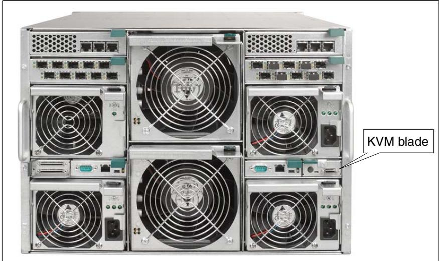
Figure 65: Position of the KVM blade
