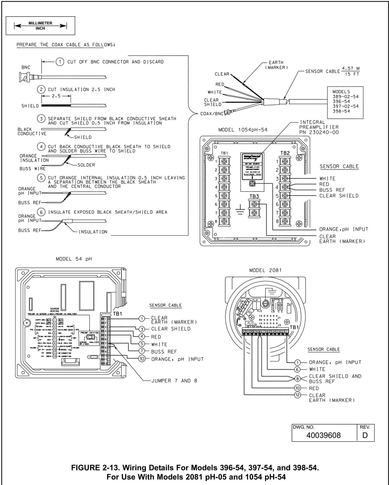
**FIGURE 2-13. Wiring Details For Models 396-54, 397-54, and 398-54.
