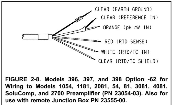
FIGURE 2-8. Models 396, 397, and 398 Option -62 for Wiring to Models 1054, 1181, 2081, 54, 81, 3081, 4081, SoluComp, and 2700 Preamplifier (PN 23054-03). Also for use with remote Junction Box PN 23555-00.
