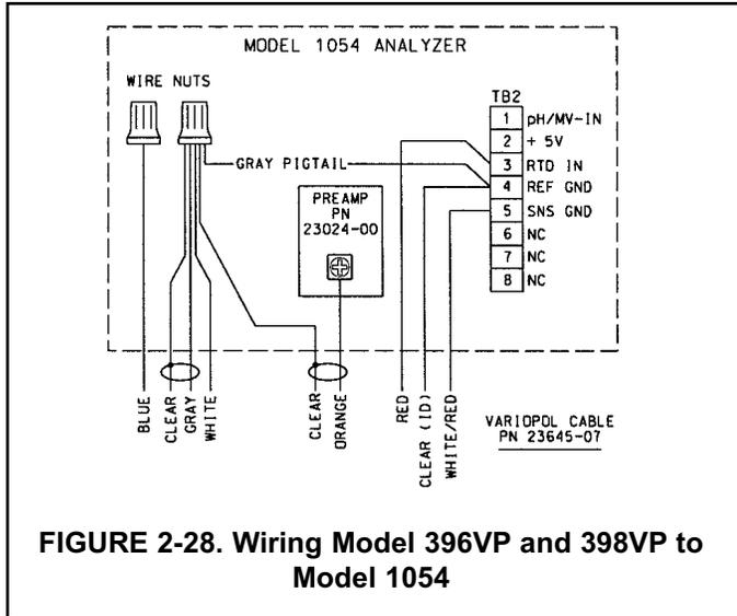
**FIGURE 2-28. Wiring Model 396VP and 398VP to Model 1054**
