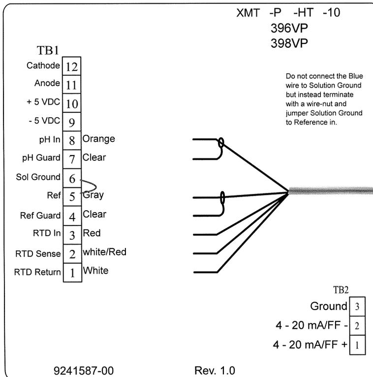
**FIGURE 2-38. Wiring Models 396VP & 398VP to Model Xmt-P-HT-10**
