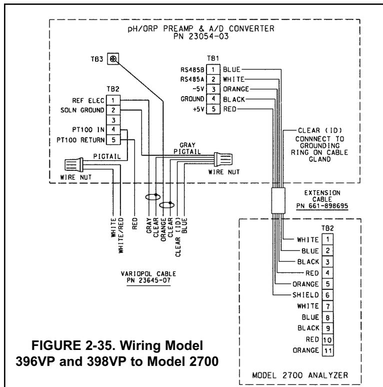
FIGURE 2-35. Wiring Model 396VP and 398VP to Model 2700
