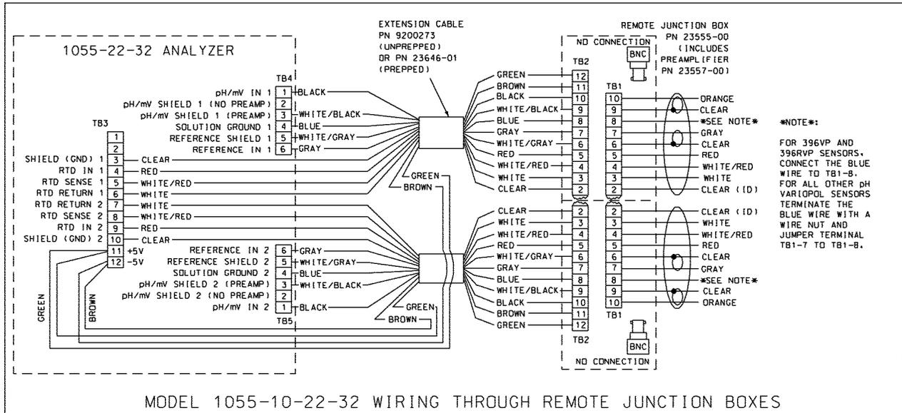
**FIGURE 2-36. Wiring Model 396VP-54 to Model 1055-22-32**
