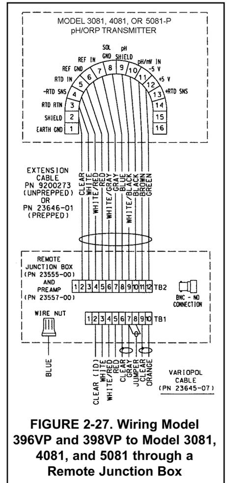
**FIGURE 2-27. Wiring Model 396VP and 398VP to Model 3081, 4081, and 5081 through a Remote Junction Box**
