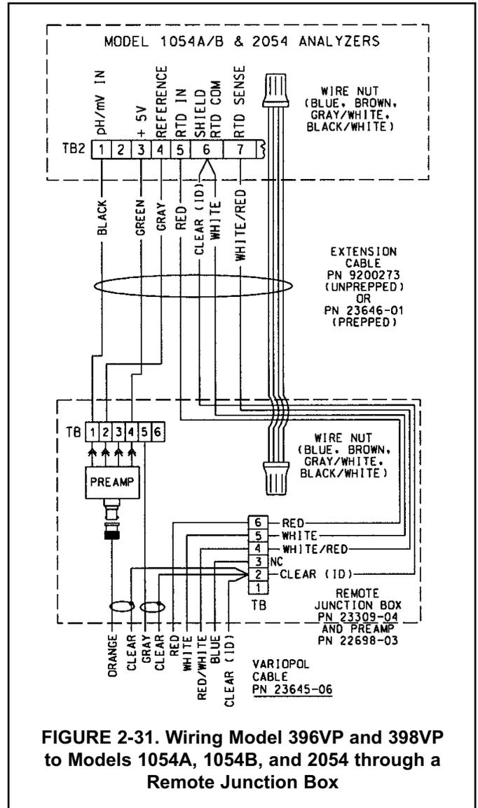
**FIGURE 2-31. Wiring Model 396VP and 398VP to Models 1054A, 1054B, and 2054 through a Remote Junction Box**
