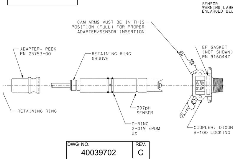
NOTE: The EP gasket (see drawing #40039702) provided with the coupler should be periodically inspected. If gasket shows signs of corrosion, replacement will be necessary to ensure a proper and secure seal between the coupler and adapter.
