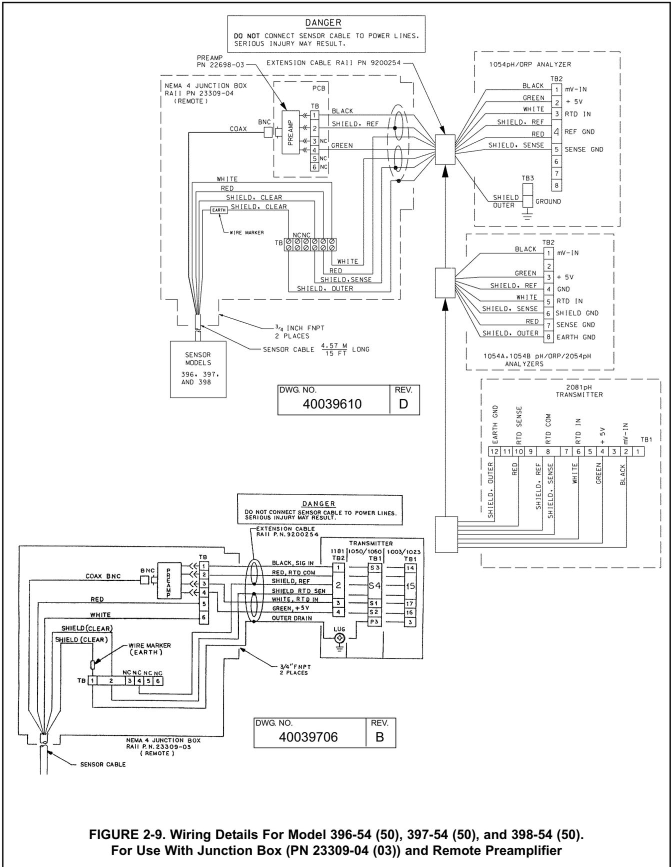
**FIGURE 2-9. Wiring Details For Model 396-54 (50), 397-54 (50), and 398-54 (50).
