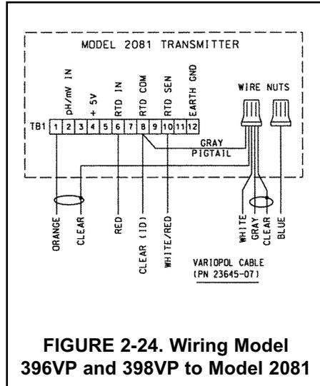
**FIGURE 2-24. Wiring Model 396VP and 398VP to Model 2081**
