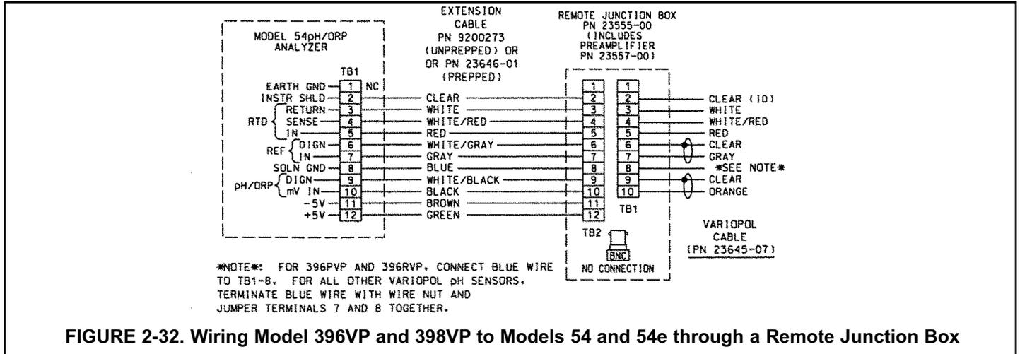
FIGURE 2-32. Wiring Model 396VP and 398VP to Models 54 and 54e through a Remote Junction Box
