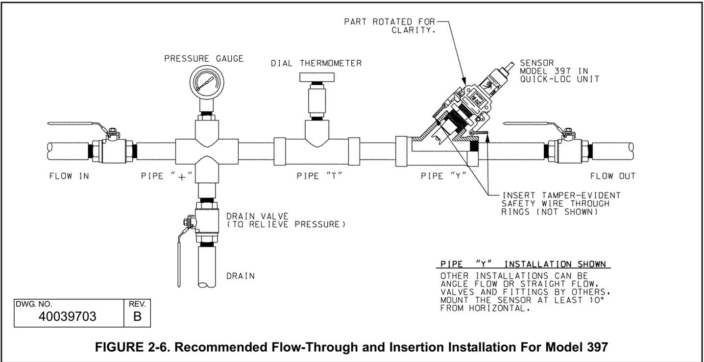
FIGURE 2-6. Recommended Flow-Through and Insertion Installation For Model 397
