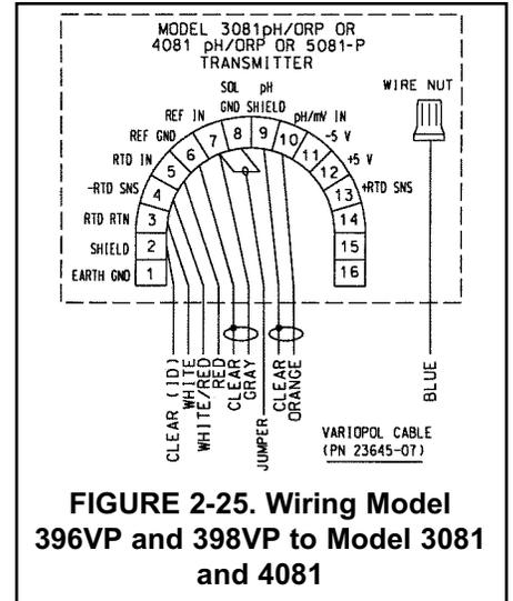
**FIGURE 2-25. Wiring Model 396VP and 398VP to Model 3081 and 4081**
