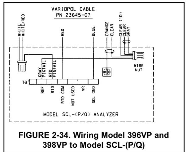
FIGURE 2-34. Wiring Model 396VP and 398VP to Model SCL-(P/Q)
