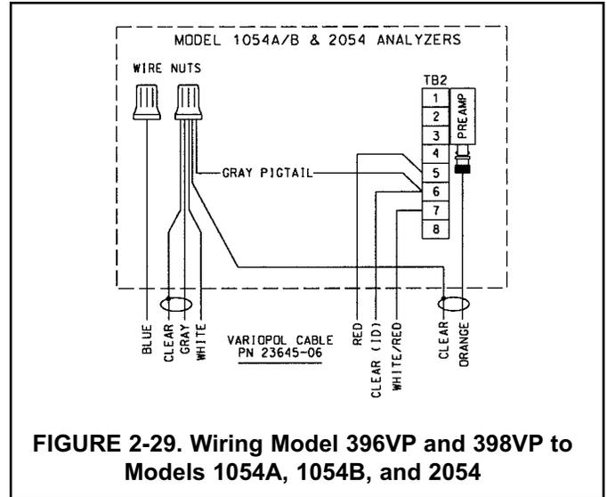
**FIGURE 2-29. Wiring Model 396VP and 398VP to Models 1054A, 1054B, and 2054**
