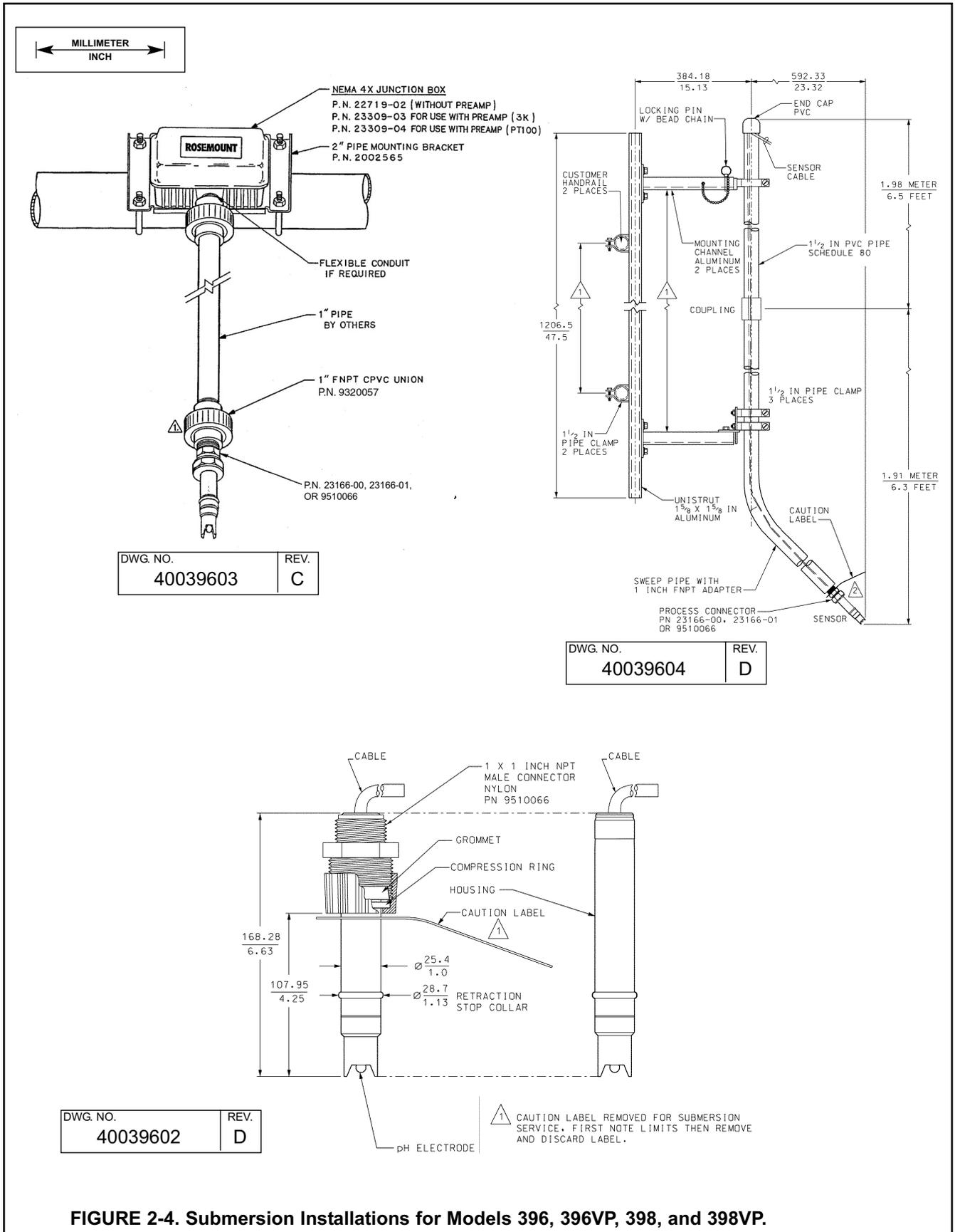
FIGURE 2-4. Submersion Installations for Models 396, 396VP, 398, and 398VP.
