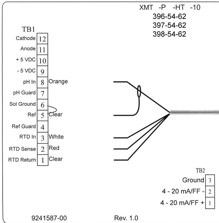
**FIGURE 2-37. Wiring Models 396-54-6, 397-54-62, & 398-54-62 to Model Xmt-P-HT-10**
