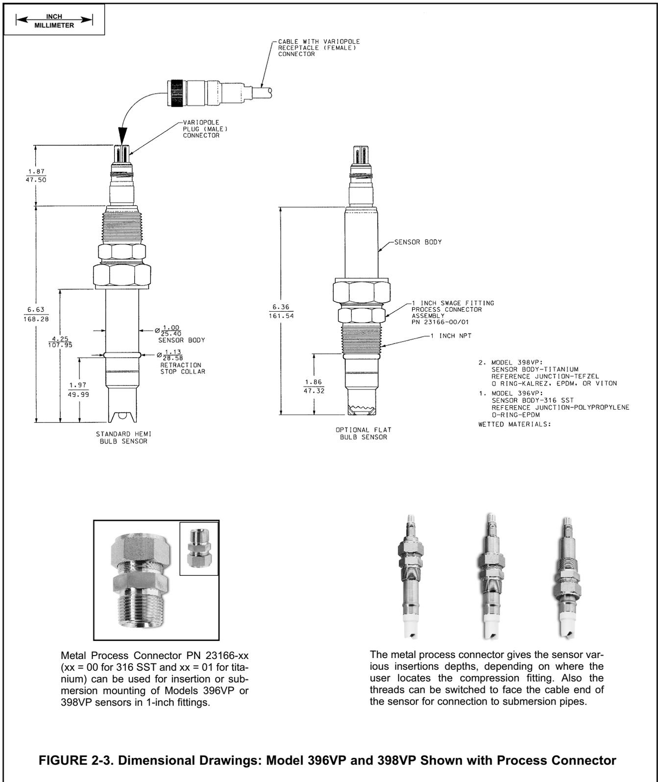
FIGURE 2-3. Dimensional Drawings: Model 396VP and 398VP Shown with Process Connector
