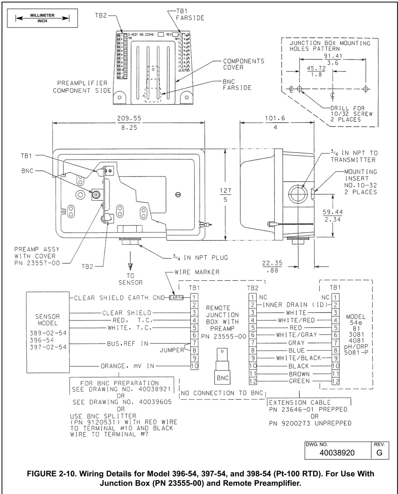
FIGURE 2-10. Wiring Details for Model 396-54, 397-54, and 398-54 (Pt-100 RTD). For Use With Junction Box (PN 23555-00) and Remote Preamplifier.
