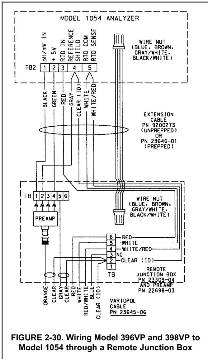
**FIGURE 2-30. Wiring Model 396VP and 398VP to Model 1054 through a Remote Junction Box**
