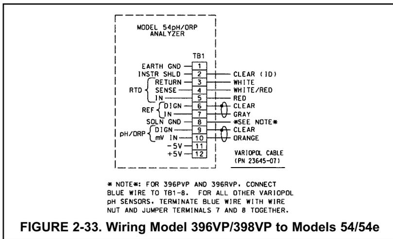
FIGURE 2-33. Wiring Model 396VP/398VP to Models 54/54e
