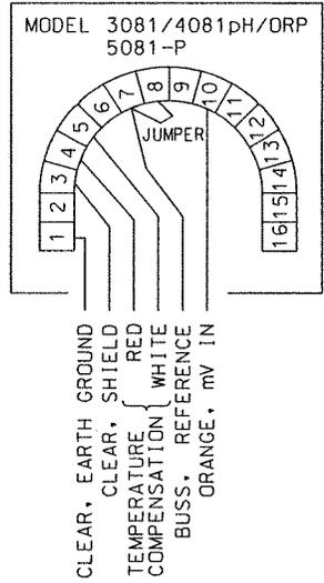
NON-DIAGNOSTIC pH SENSOR WITHOUT PREAMPLIFIER AND SOLUTION GROUND
