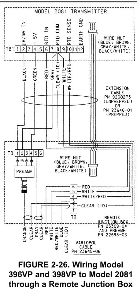
**FIGURE 2-26. Wiring Model 396VP and 398VP to Model 2081 through a Remote Junction Box**
