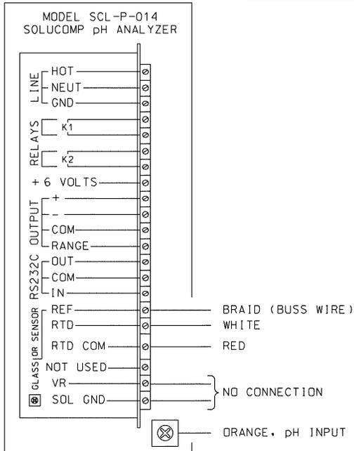
1. CUT OFF THE CLEAR SHIELD AND CLEAR EARTH WIRES BEFORE CONNECTING THE SCL-P-014 TERMINALS.
