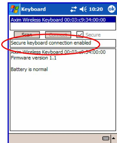
12. If the connection process is successful, the **Secure keyboard connection enabled** message will display on the Pocket PC device. This is the normal mode for wireless communication between the Axim™ Wireless keyboard and the Pocket PC device during use.
