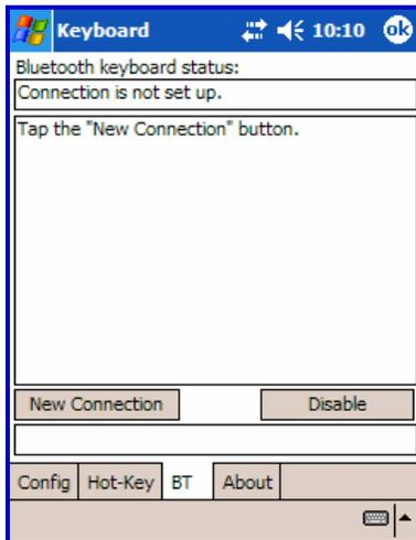
4. The **New Connection** window is used to connect the Pocket PC device to the Axim™ Wireless keyboard. Tap **New Connection** to begin the process.
