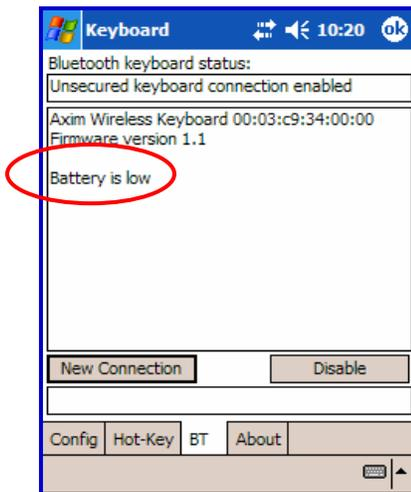
14. On the **Bluetooth Status Page** the keyboard battery information is displayed. The three states of the battery are:
