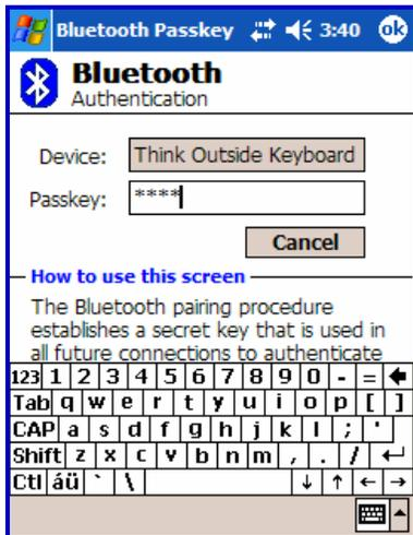
10. If you choose a secure connection by checking the **Secure** box, the Pocket PC Bluetooth system software will prompt you for a passkey. You are likely to see the **Bluetooth Passkey** dialog shown here, but this is variable by device. Enter a passkey using the Pocket PC on-screen keyboard, then tap OK in the top right corner of the window. Type the same passkey number on the Axim™ Wireless keyboard, using **Left <Fn> + <Number>** keys. When finished, press the <Enter> key.
