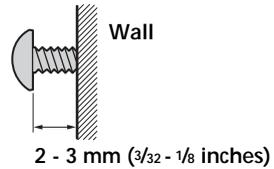
**2** Press bracket (A) to the wall and slide it down. Then fully tighten the four screws on the wall.
