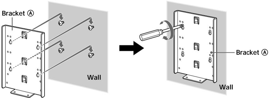
**3** Fully tighten four of the screws you prepared in screw holes (1) to (4) firmly.
