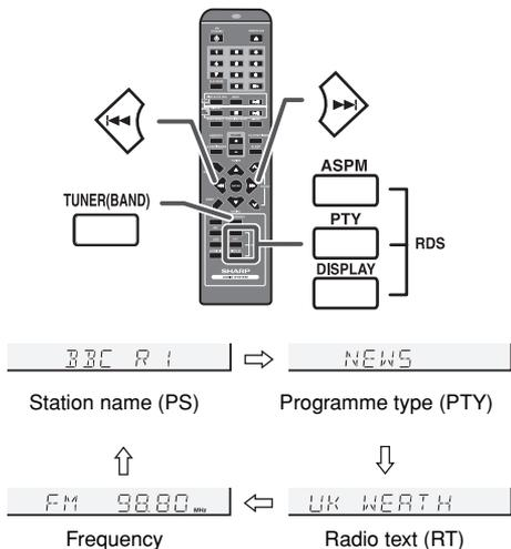
When tuning in to a station other than an RDS station or to an RDS station which sends weak signal, the display will change in the following order:
