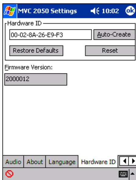
The Hardware ID is generated by reading MAC addresses from the PDA NIC. When the MVC 2050 is used with most server types, the Hardware ID it uses must be unique. Some software, such as VPN client software, creates artificial network interfaces with MAC addresses that are common to all installations of the software. As a result, the MAC address is the same on many different computers.
