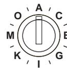
You can operate two or more independent Plug 'N Power systems in your home by using a different house code for each system. Of course, each system must have its own controller and modules.
