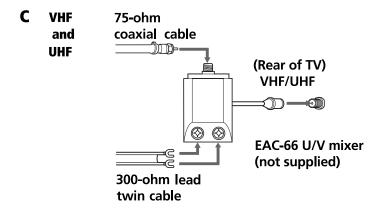
This allows you to connect your TV to both a cable system and a dipole antenna, in order to view both cable and local channels.
