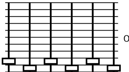
Below is the worst sort of curve to use because you are using EQ to *add volume*. With exaggerated boost you can easily run your power amplifiers into "clipping" (see page 6) and damage your speakers.
