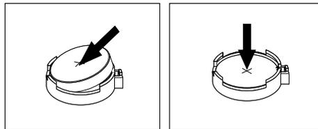
Figure 31. Installing a new battery
