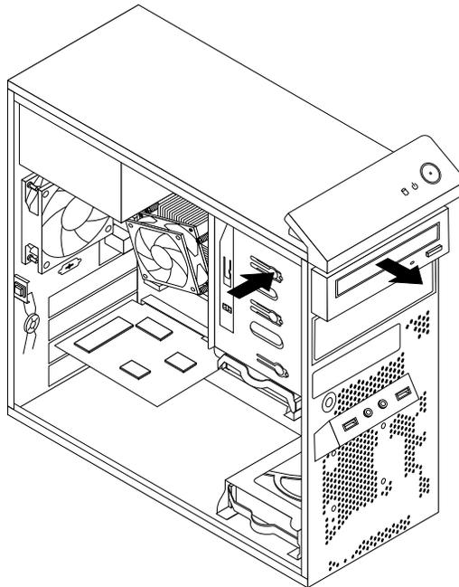
*Figure 19. Removing the optical drive*
