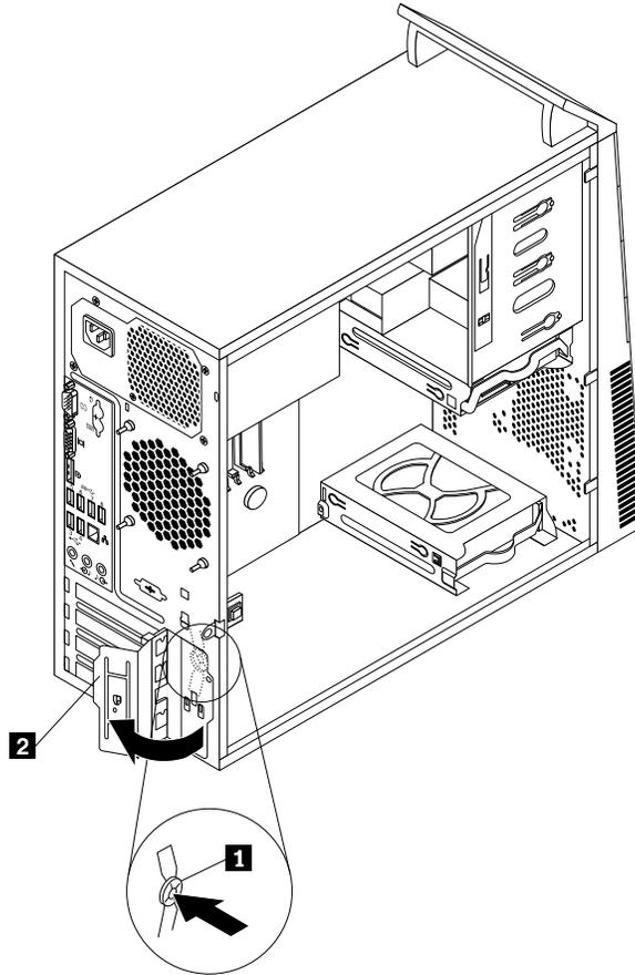
Figure 13. Opening the PCI card latch
