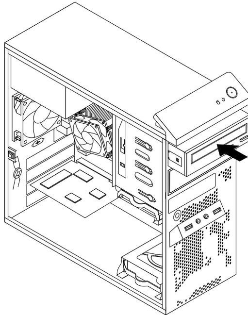
Figure 21. Installing the optical drive
