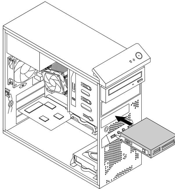
Figure 25. Installing the card reader
