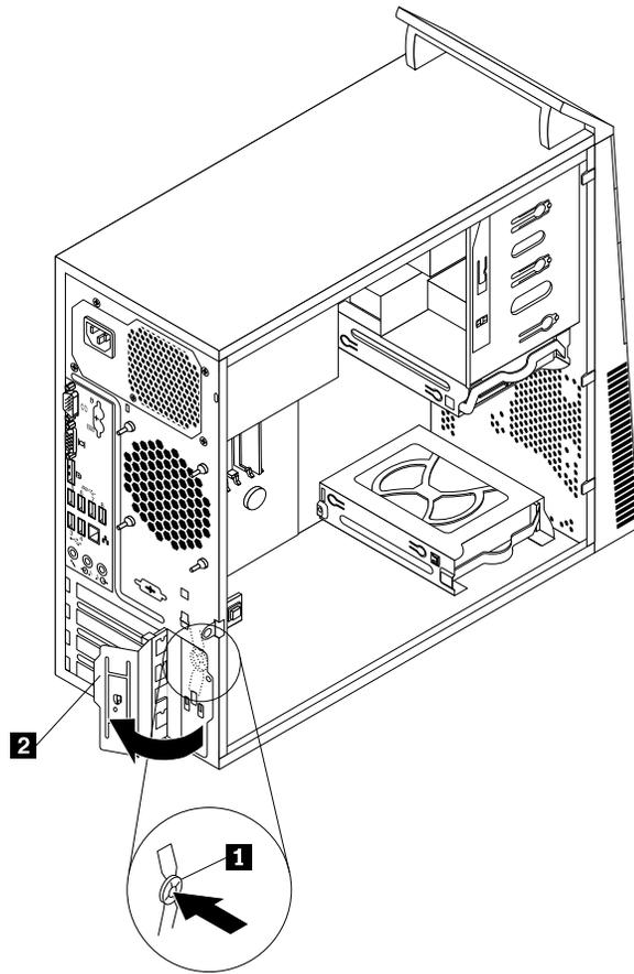
Figure 66. Opening the PCI card latch
