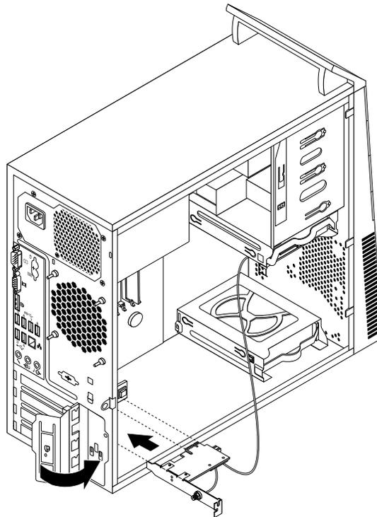
Figure 73. Installing the WiFi adapter card
