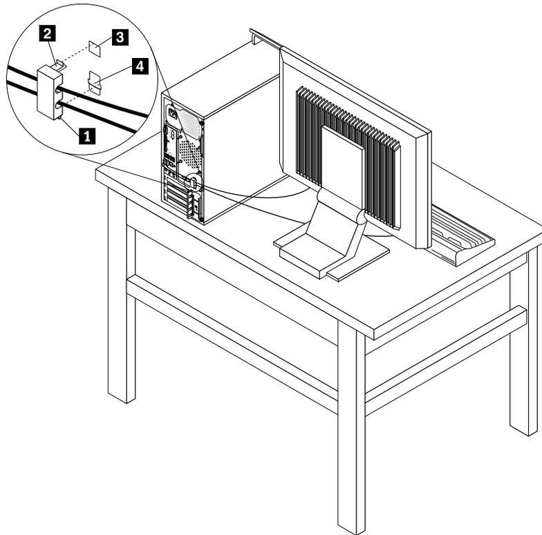
Figure 9. Installing a cable lock
