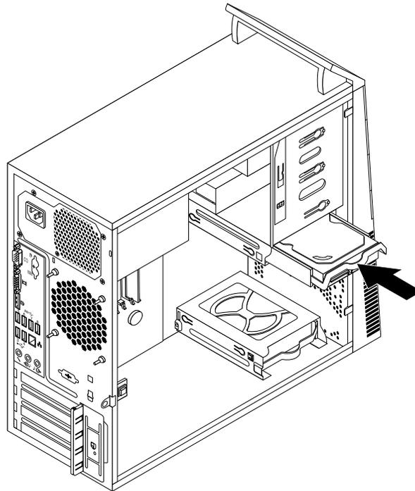
Figure 50. Installing the primary hard disk drive
