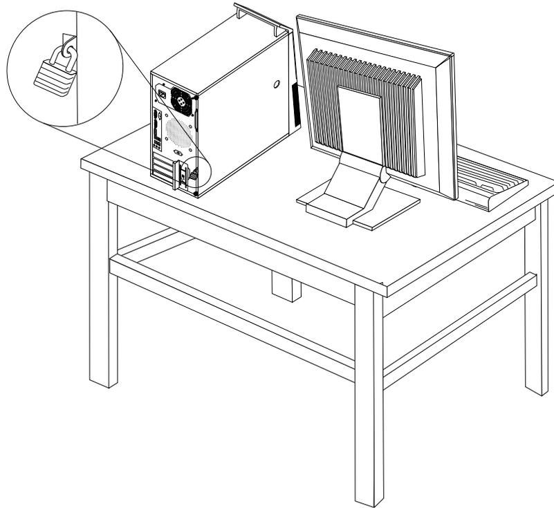
*Figure 8. Installing a padlock*
