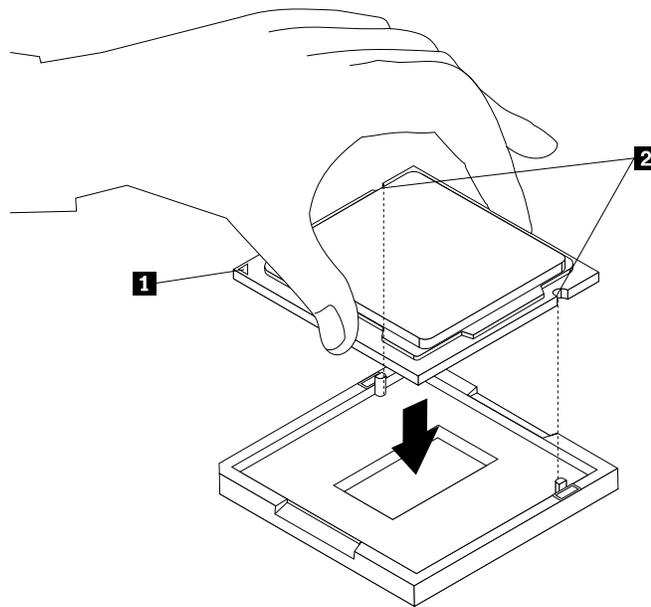
Figure 36. Installing the microprocessor
