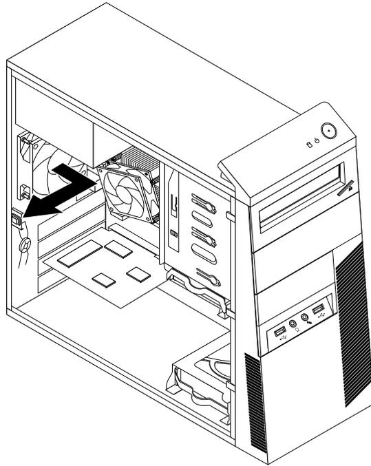
*Figure 56. Removing the rear fan assembly*
