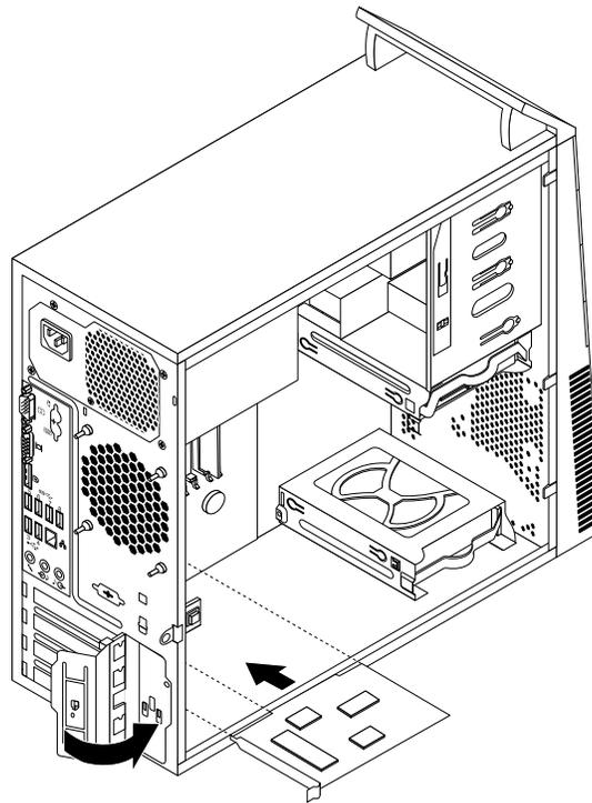
Figure 15. Installing a PCI card
