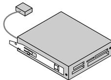
Figure 28. Installing the card reader retainer
