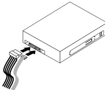
Figure 22. Connecting the optical drive
