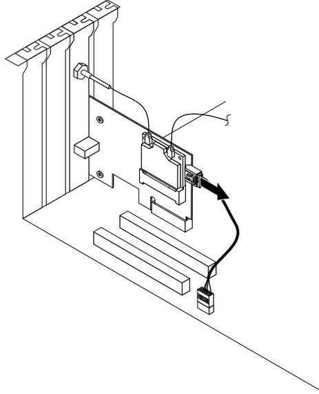
*Figure 65. Disconnecting the Bluetooth cable*
