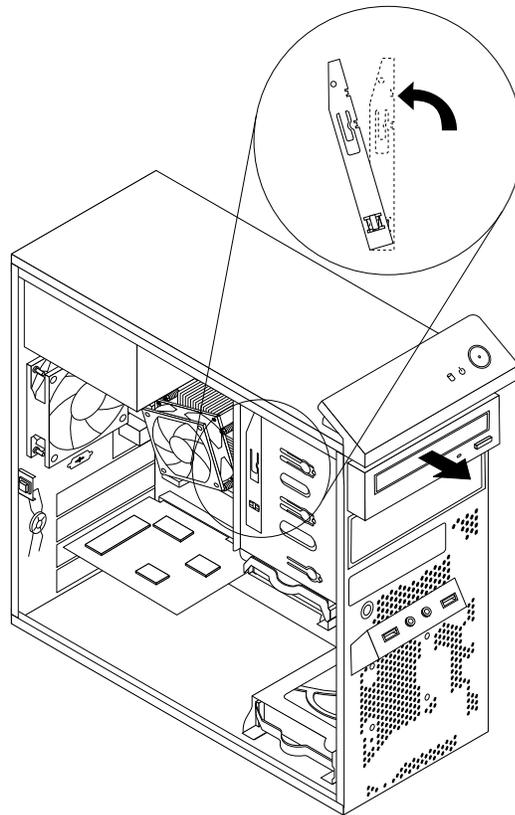
Figure 23. Removing the card reader retainer
