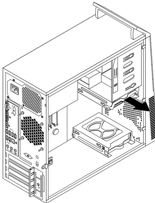
Figure 48. Removing the primary hard disk drive
