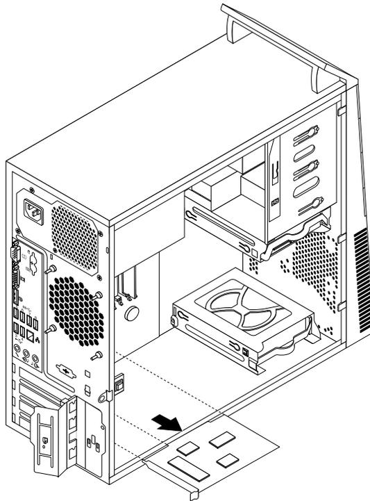
Figure 14. Removing a PCI card
