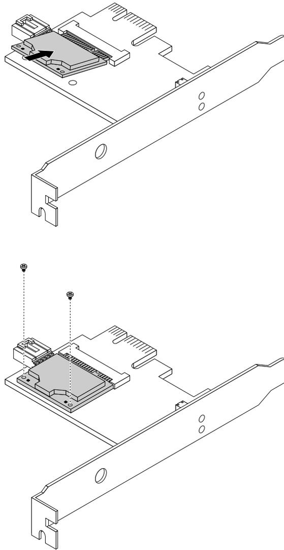
Figure 71. Installing the WiFi card module
