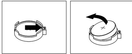
Figure 30. Removing the old battery
