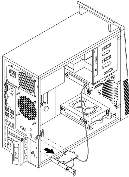
Figure 67. Removing the WiFi adapter card
