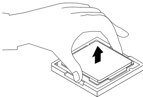
Figure 35. Removing the microprocessor
