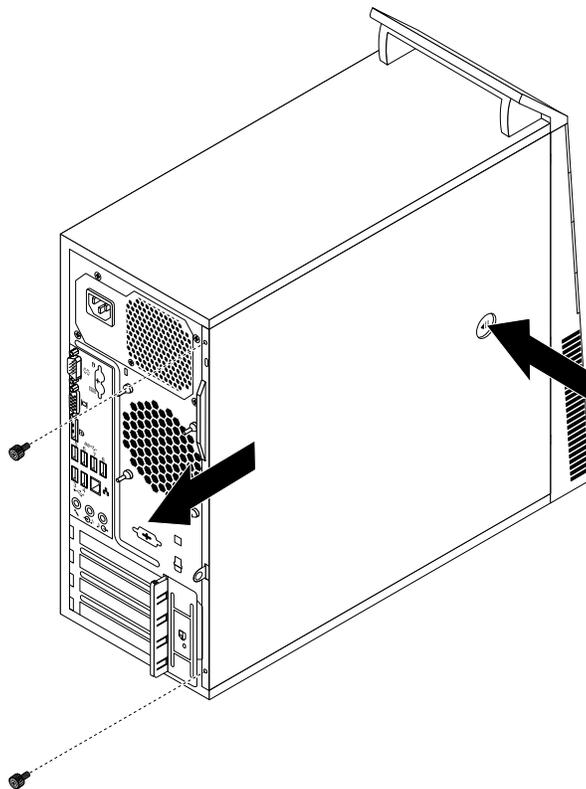
Figure 11. Removing the computer cover
