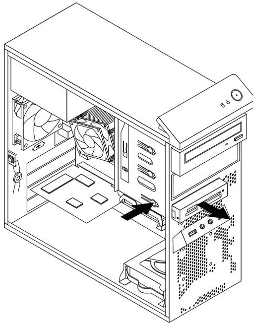
Figure 27. Removing the card reader
