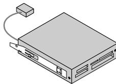
Figure 24. Installing the card reader retainer
