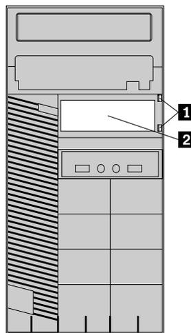
Figure 26. Removing the card reader cover
