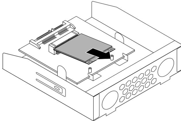
*Figure 44. Removing the mSATA solid state drive*
