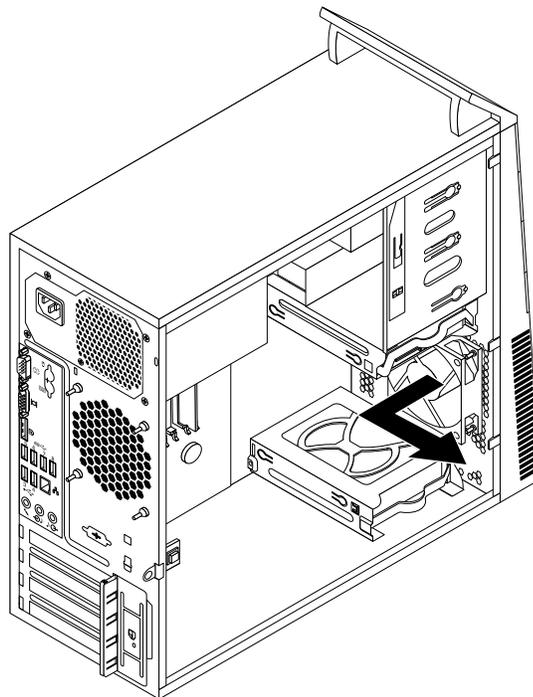
Figure 54. Removing the front fan assembly
