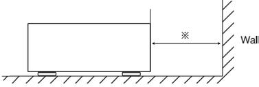
**Do not block ventilation openings or stack other equipment on the top.**
