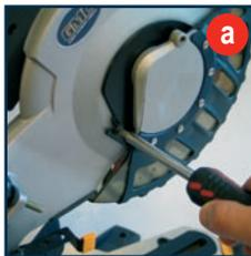
6. Pull the rotating blade guard (12) down then swing it up together with the blade bolt cover (14). When the rotating blade guard (12) is positioned over the upper fixed blade guard (9) it is possible to access the blade bolt (Fig. b).
