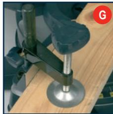
Use the clamp assembly lock (11) at the back of the fence to secure the clamp assembly in position (Fig. H).
