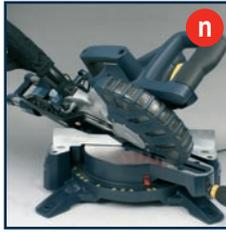
Use the slide action when cutting wide workpieces.
