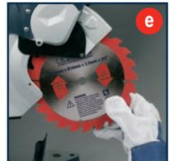
**CAUTION.** To ensure correct blade rotation, always install the blade with the blade teeth and the arrow printed on the side of the blade pointing down. The direction of blade rotation is also stamped with an arrow on the upper blade guard.
