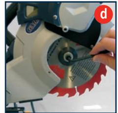
9. Remove the flat washer and outer blade washer and the blade.
