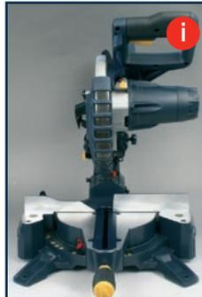
1. Pull on the release knob (6) and lift the saw arm (5) to its full height.
