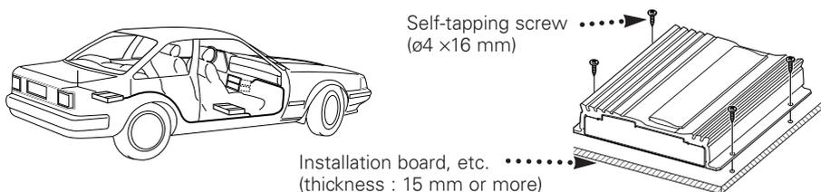
Since the power amplifier has no parts which require operation, it can be installed at a position away from the driver's seat without any hindrances.
