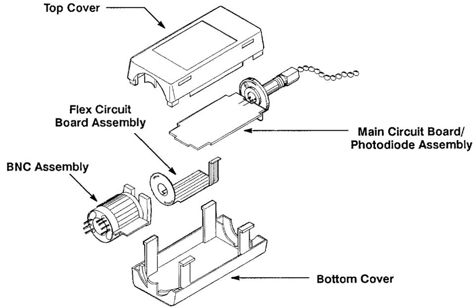
**Figure 6-2: Assembly Replacement**
