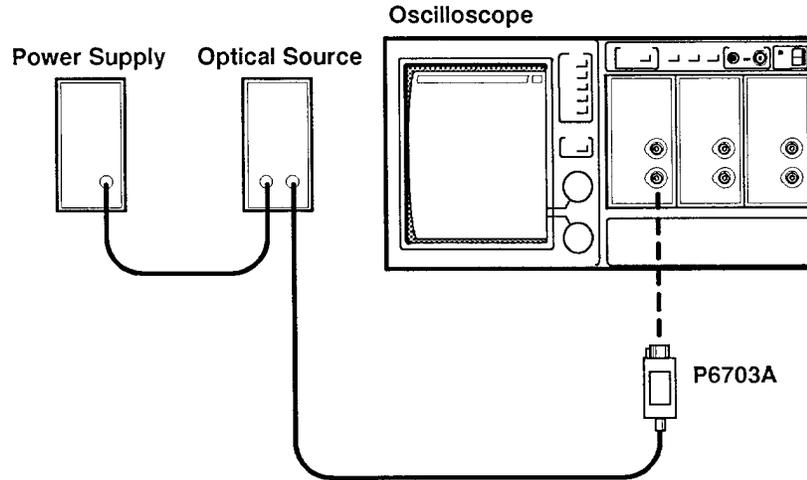
Figure 4-1: Conversion Gain and Offset Gain Check Setup
