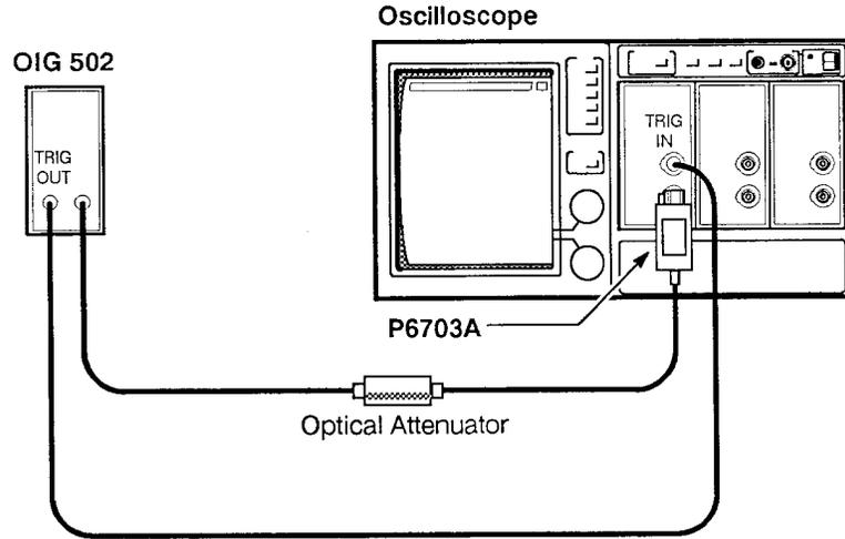
**Figure 4-2: Bandwidth Check Setup**
