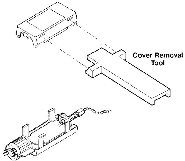
**Figure 6-1: Top Cover Removal**
