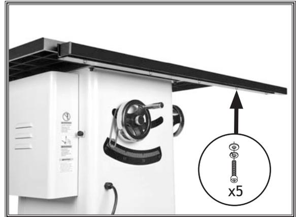
Figure 20. Fence rail tube attached.
