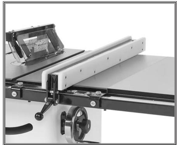
Figure 21. Fence assembly installed.
