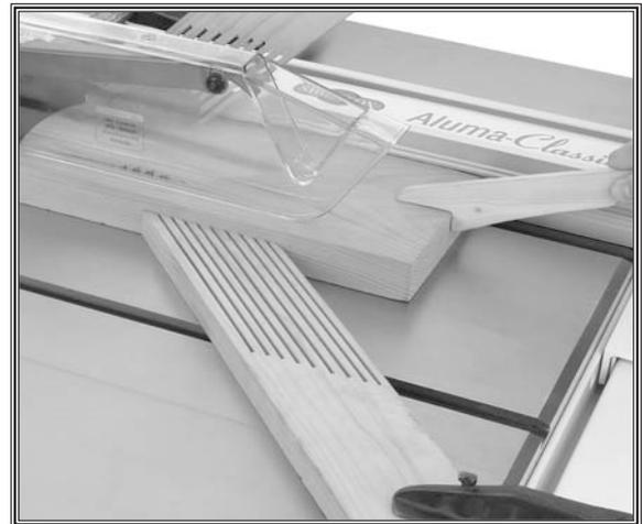
Figure 45. Example photo of a ripping operation.
