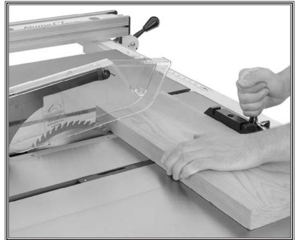
**Figure 46.** Example photo of a crosscutting operation.
