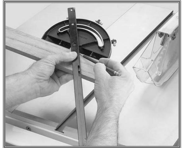
**Figure 47.** Example photo of making a miter mark.
