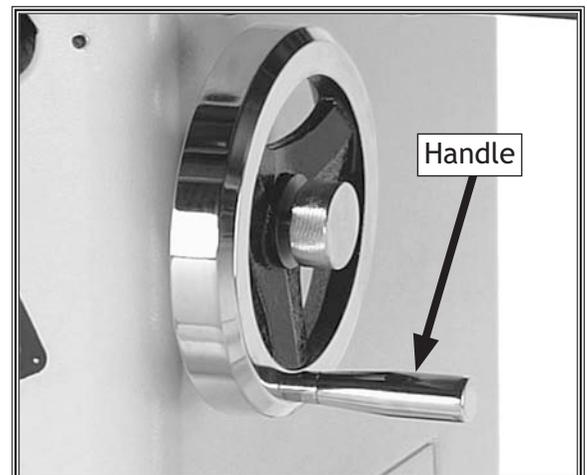
**Figure 13.** Handwheel handle installed.
