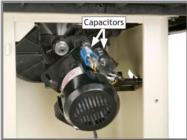
Figure 110. Motor capacitor location.
