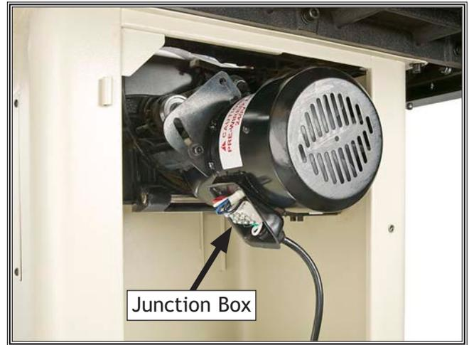
Figure 111. Motor junction box location.
