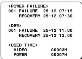
POWER FAILURE . . . . The number of power failures, and the date and time of the most recent power failure and recovery are displayed.
