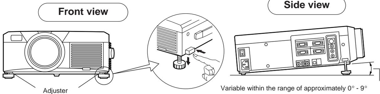
1. Lift up the projector and release the adjuster lock.
