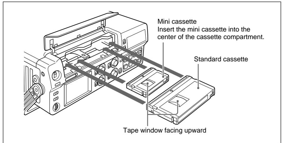
The cassette is automatically loaded into the unit.
