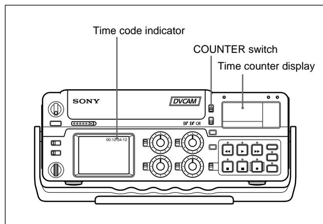
Use the COUNTER switch to select the type of time data to be displayed.
