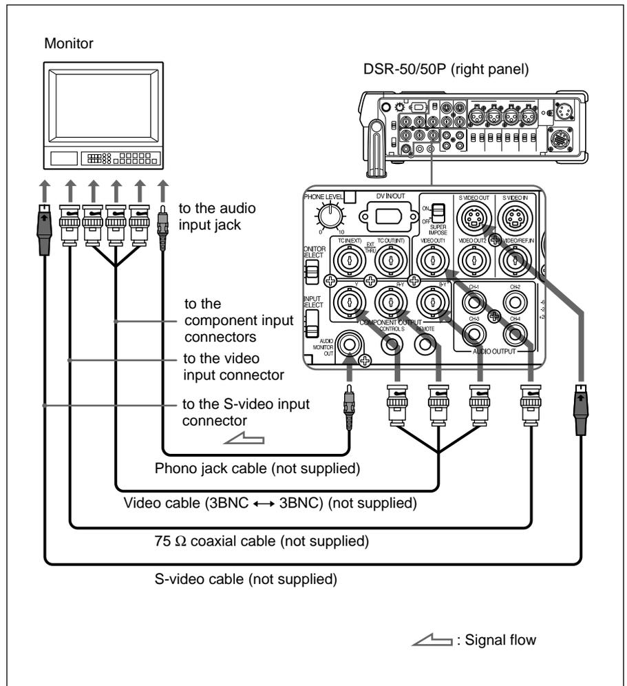
Connect one of the followings as a video cable; video cable (3BNC ↔ 3BNC), 75 Ω coaxial cable, or S-video cable.
