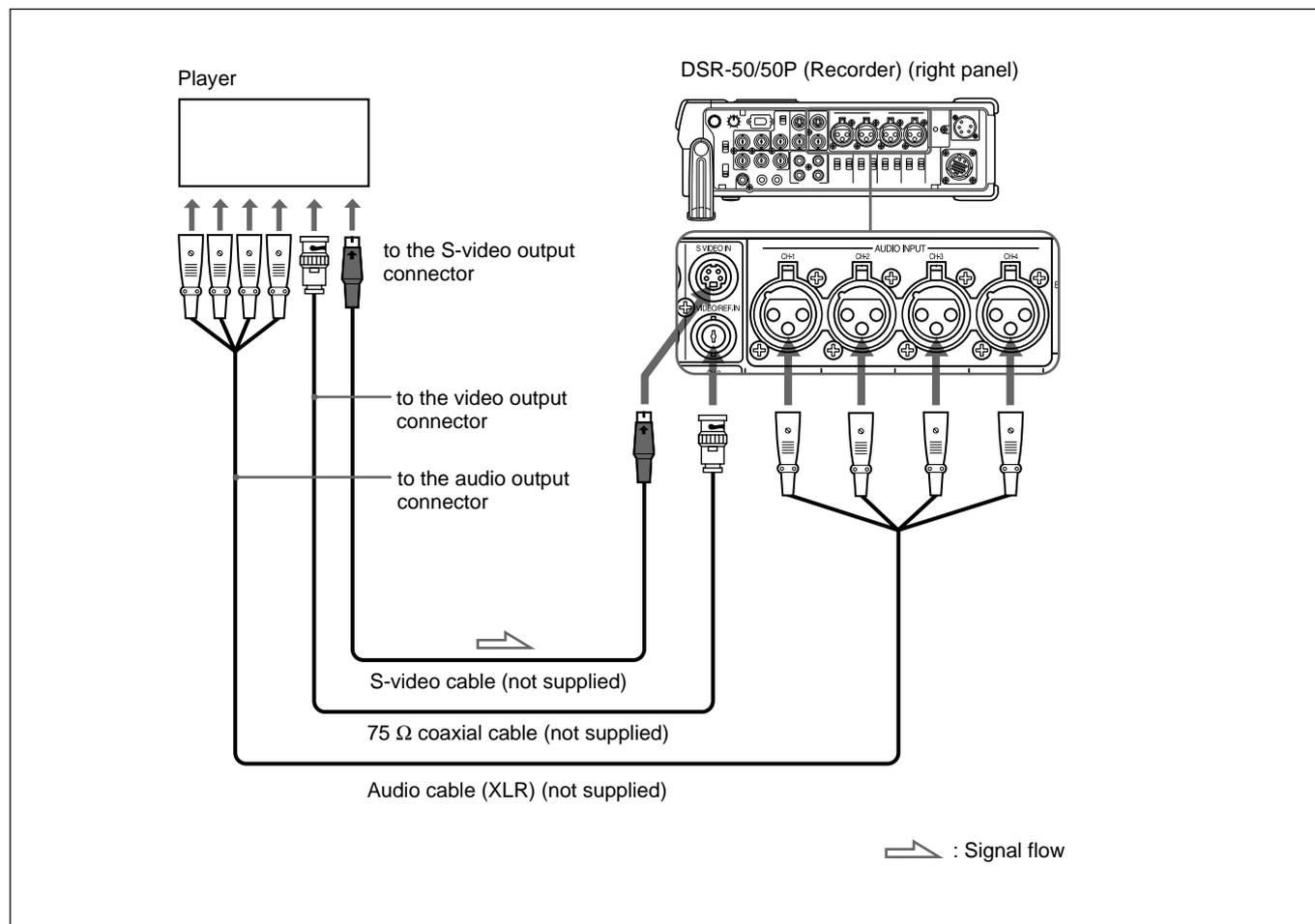
Connect one of the followings as a video cable; S-video cable or 75  $\Omega$  coaxial cable.
