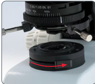
Close the Koehler field diaphragm
