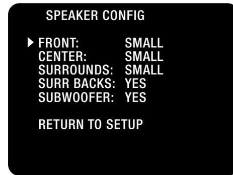
In order to optimize the performance of your system, the GTP-860 II can be configured specifically for the speakers in your system. Information about each of your speakers allows the GTP860 II to tailor the audio output for best sound. The setup procedure breaks your speaker system into five groups: front, center, surrounds, surround backs and subwoofer. There are a few options for each group.
