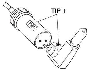
If you use the special Dell plug, align **TIP** on the Dell plug with **TIP** marked on the output socket. ✓
