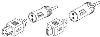
4. Insert the Adaptaplug into the device to be powered, then insert
