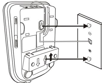
4. Put the phone over the wall plate, make sure both posts fit into slots on the back of the phone. Then slide the phone down to lock the phone into the wall plate.
