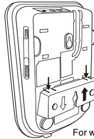
For wall mounting, install bracket with this arrow facing up and install bracket on lower part of phone
