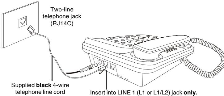
To connect two single-line telephone jacks
