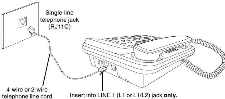
For this connection, you can only use LINE 1 and no need to use the AC adaptor if you have installed the batteries.
