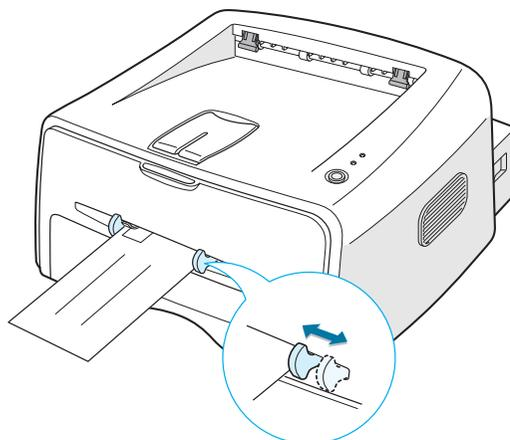
**3** When you print on envelopes, you must select **Manual Feed** for **Source** from the software application, and then select the correct paper size and type. For details, see page 4.6.
