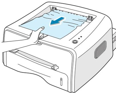
When you pull the jammed paper, if there is resistance and the paper does not move immediately, stop pulling. Continue with the next step.
