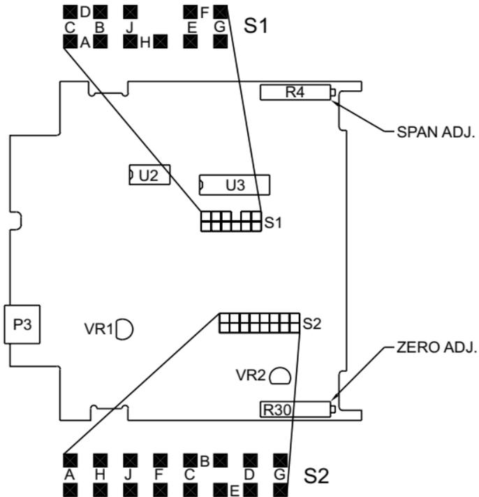
Figure 5-1 Main Board Jumper Locations
