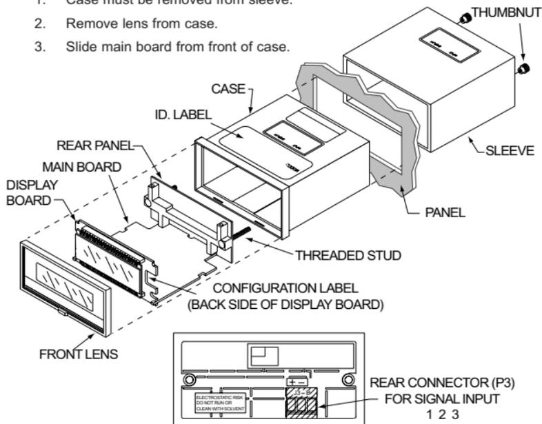
Figure 3-1 Exploded View (includes rear panel)
