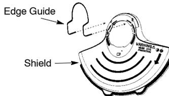
2. Align the installation arrow on the shield with the installation arrow on the motor housing (see illustration below).
