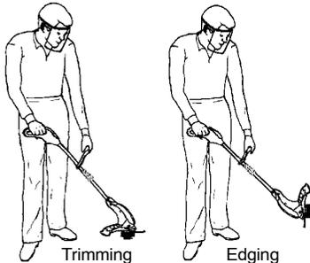
**⚠ WARNING:** Always wear eye protection. Never lean over the trimmer head. Rocks or debris can ricochet or be thrown into eyes and face and cause blindness or other serious injury.
