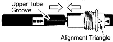
2. Try to pull tubes back apart. If the tubes do not come apart, they are properly snapped into place. If the tubes come apart, repeat step 1 and push until the tubes snap into place.
