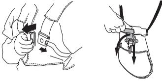
Check that the harness straps are correctly positioned. Once the harness and machine have been adjusted, check that the harness quick release works correctly.
