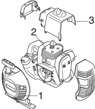
The cooling system consists of:
