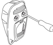
If the muffler on your machine is fitted with a spark arrestor screen this must be cleaned regularly. A blocked screen will cause the engine to overheat and may lead to serious damage.
