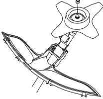
When fitting, tighten the nut in the opposite direction to the direction of rotation of the cutting attachment. To remove it, undo the nut in the same direction as the cutting attachment rotates. (CAUTION! The nut has a left-hand thread.) Tighten the nut using the socket spanner.
