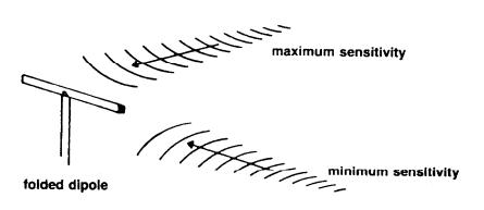
The dipole antenna rapidly looses its effectiveness when rolled up or carelessly dropped behind a cabinet, etc. If the "T" antenna is undesirable from a functional or decor point of view, your ADCOM dealer will be pleased to show you a variety of indoor antennas that might be more appropriate. We do suggest, however, that you ask for a home trial as reception conditions vary enormously from location to location.
