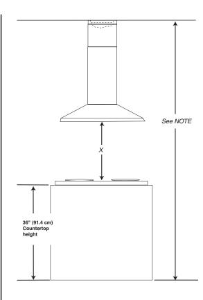
Note: The hood chimneys are adjustable and designed to meet varying ceiling or soffit heights depending on the distance "X" between the bottom of the hood and the cooking surface. For higher ceilings, a 40" (101.6 cm) Chimney Extension Kit Part Number 8212698 (Black), Kit Part Number 8212696 (Stainless Steel) or Kit Part Number 8212697 (White) is available. See your dealer. The chimney extension replaces the upper chimney shipped with the hood.
