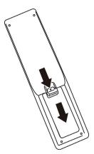
2 Insert two AAA batteries into the battery compartment. Make sure that you match the + and – symbols on the batteries with the + and – symbols in the battery compartment.
