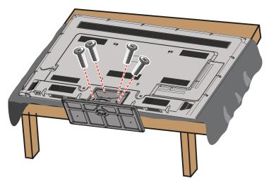
3 Insert the four provided spacers into the mount screw holes on the back of your TV.
