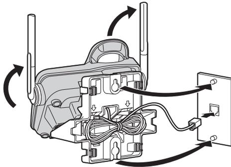
**To remove the wall mounting adaptor**
