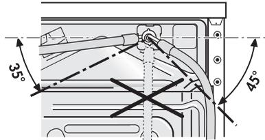
2. Connect the hose with the straight connection to a water tap with a screw thread R 3/4 (inches)
